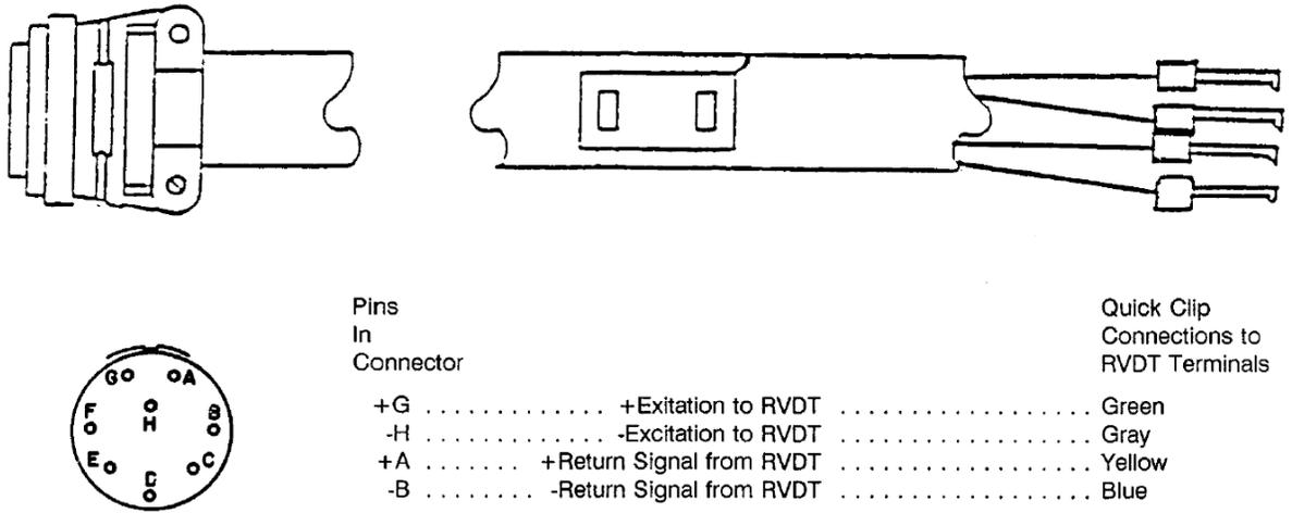
Figure 1. Cable Supplied to Connect Test Box to RVDT in Actuator
