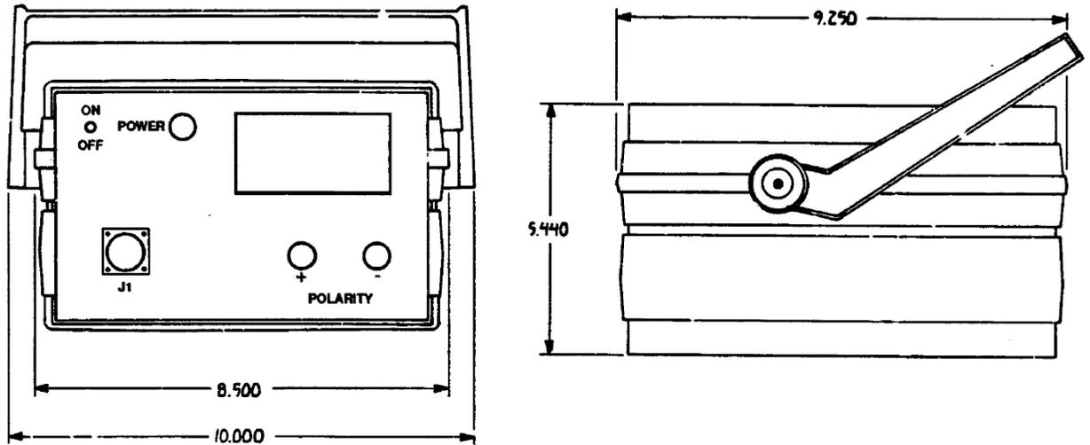
Figure 2. Outline Drawing of T87444 RVDT Check Box
