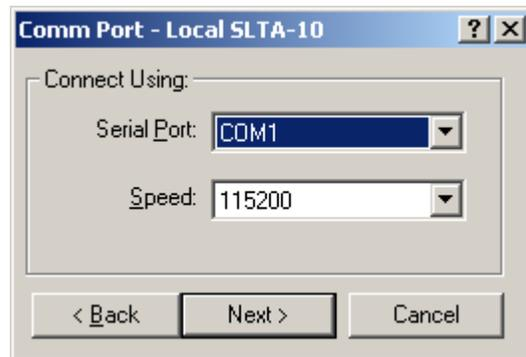
The Serial Port and Speed settings may be changed by dropdown menu at this screen. Select “Next” and “Finish” to apply the changes or select “Cancel” to ignore any changes. If the Speed setting is changed, the SLTA-10 configuration DIP switches must be changed to match the new Speed setting. Follow the table adhered to the SLTA-10 Network Adapter.
