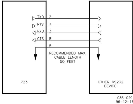
Figure A-1. 723PLUS RS-232 Connections
