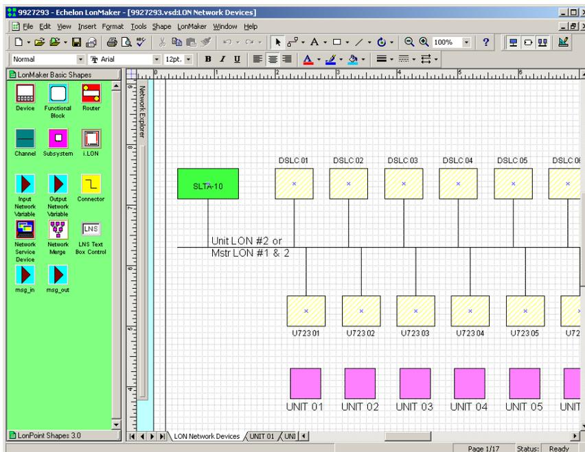
After a device is commissioned, the color changes on the drawing sheet. Devices that have been commissioned are shown with a solid green color. Devices that have not yet been commissioned are shown with a light yellow crosshatch. The drawing above shows that the SLTA-10 network interface adapter has been commissioned, but the remaining “LON Network Devices” devices have not been commissioned.
