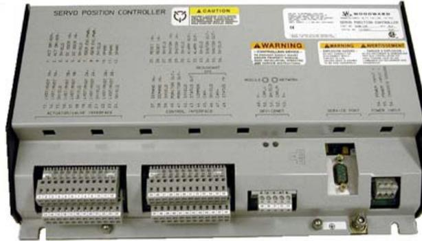
A Windows based software program is used to configure the SPC, adjust tunables, and monitor parameters via a personal computer. For ease of service, SPC configurations can be done while connected or disconnected to the unit. Once a configuration has been created, this program allows configurations to be uploaded and downloaded to other SPCs as desired.
