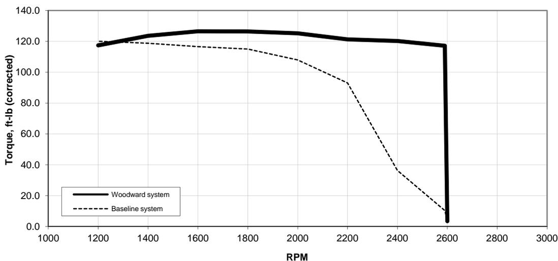
Torque vs RPM Curves (MI-04 compared to Baseline System)
