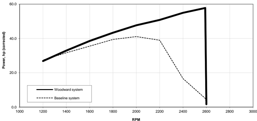
Power vs RPM Curves (MI-04 compared to Baseline System)
