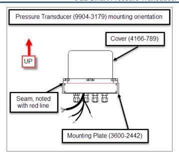
Figure R-1. Pressure Transducer Assembly Mounting Orientation
