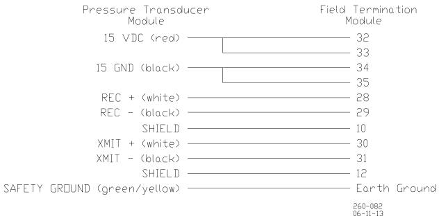
Figure 2-3. Wiring Schematic for Interface Module Port #2
