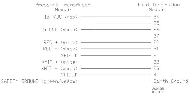
Figure 2-2. Wiring Schematic for Interface Module Port #1
