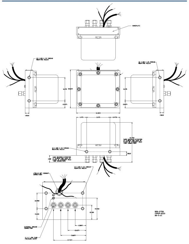
Figure 2-1. Outline Drawing of Pressure Transducer Manifold
