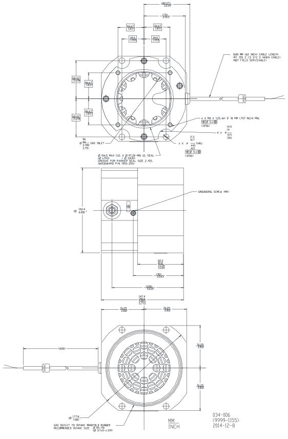
Figure 1-1. SOGAV 250 Outline Drawing (Unbalanced/Bottom-Load) (Flying Lead Version)
