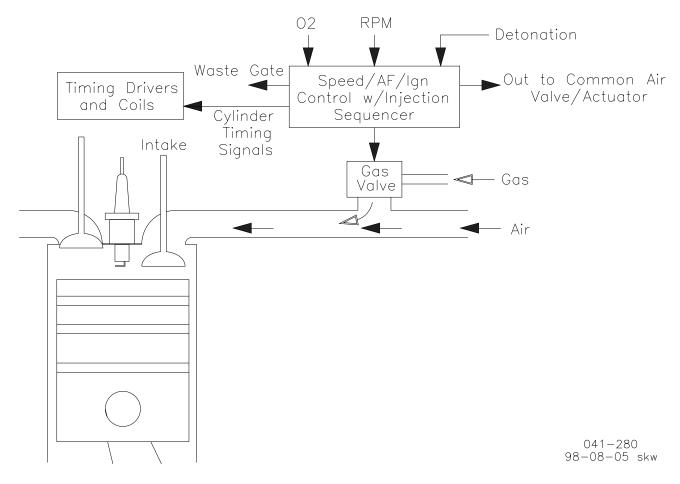
Figure 1-3. In-Manifold Electric Gas Admission
