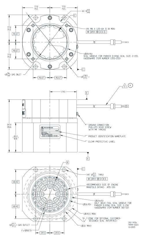
Figure 1-2a. SOGAV 250 Outline Drawing (Unbalanced/Top-Load) (Flying Lead Version)
