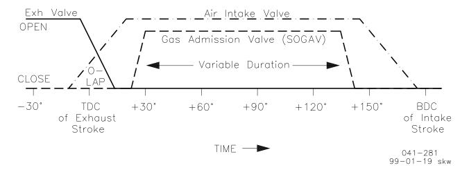
Figure 1-4. Timing: In-Manifold Gas Admission
