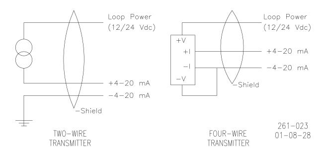
Figure 1-2a. Wiring Diagram—4–20 mA Signal
