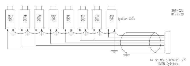
Figure 1-4. Wiring Diagram—16-Cylinder Example
