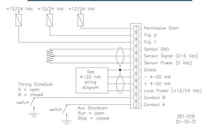
Figure 1-3. Wiring Diagram—TIS-910 Timing and Safety Controls
