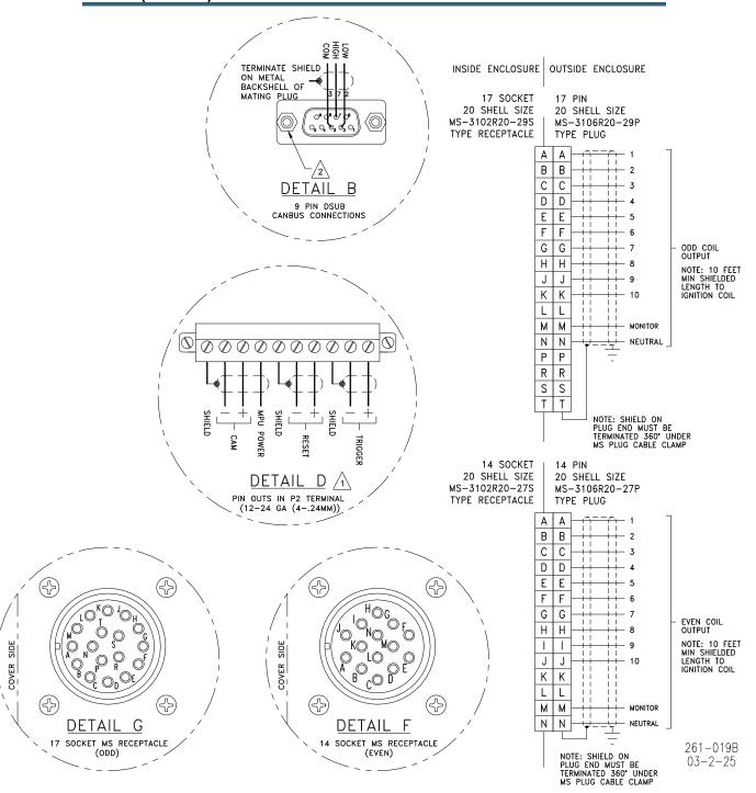
Figure 1-6b. Overall Plant Wiring Diagram
