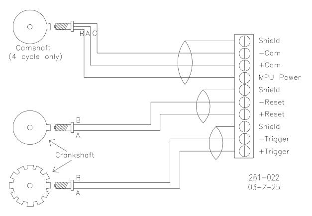
Figure 1-1. Wiring Diagram—TIS-910 Timing Sensors
