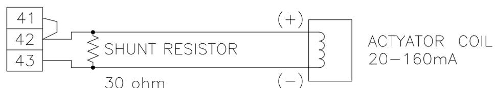
Figure 3-4. Actuator 20-160mA Shunt Resistor Connection
