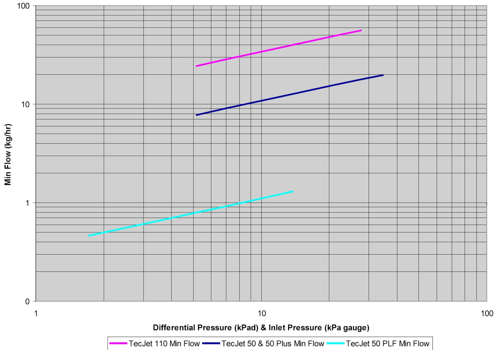
Figure 4-4. Minimum Natural Gas Flow Capacity of TecJet 50 Plus, 50 Plus PF, 50, and 110 (Natural Gas, SG=0.6, Sea Level)
