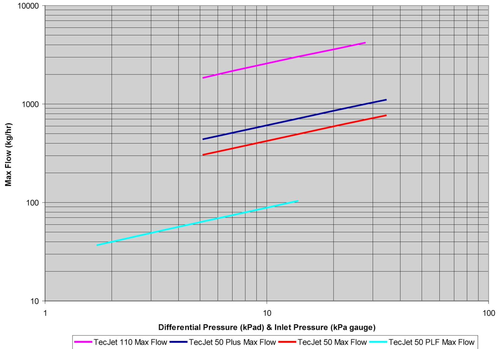
Figure 4-3. Maximum Natural Gas Flow Capacity of TecJet 50 Plus, 50 Plus PF, 50, and 110 (Natural Gas, SG=0.6, Sea Level)
