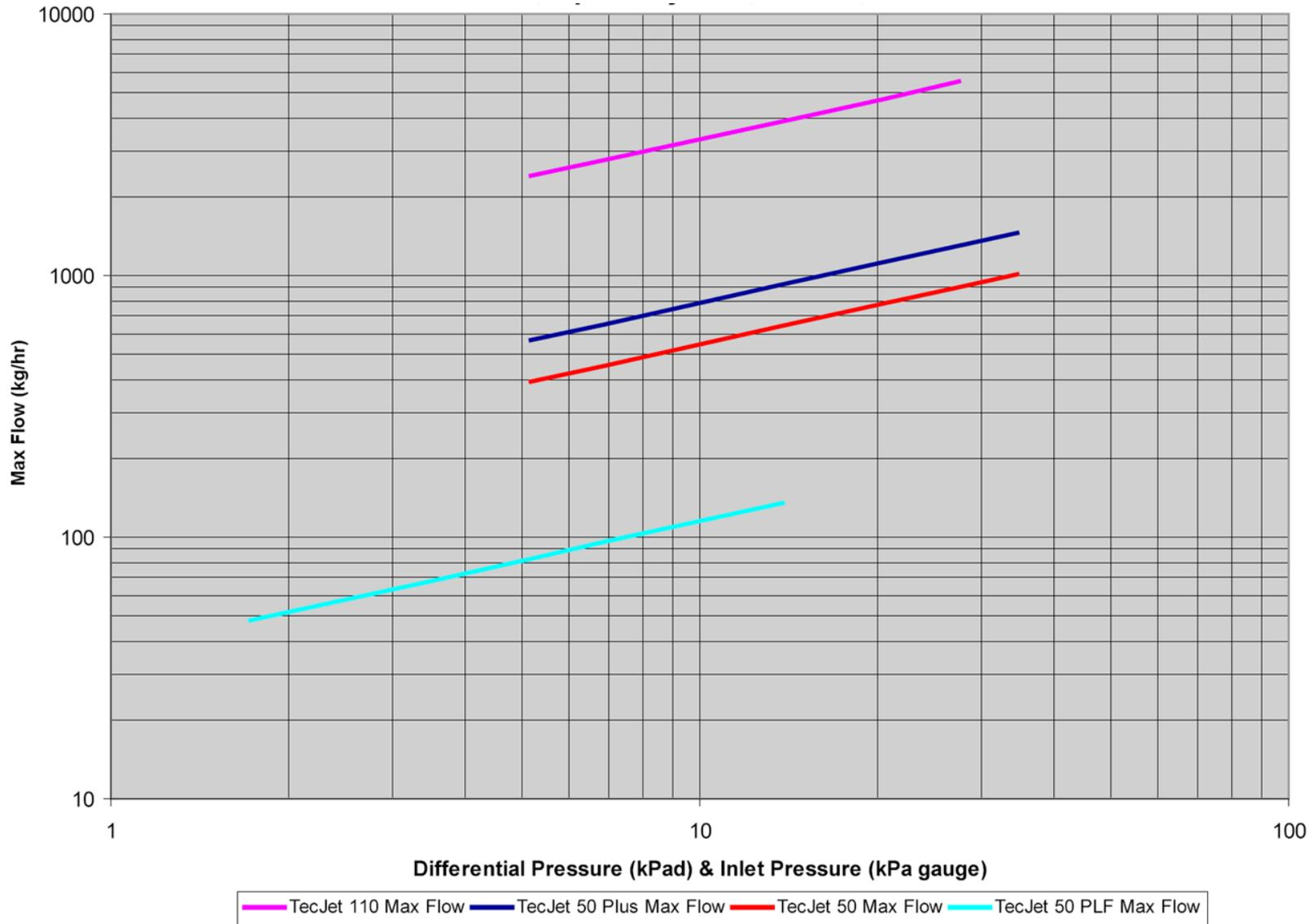
Figure 4-1. Maximum Specialty Gas Flow Capacity of TecJet 50 Plus, 50 Plus PF, 50, and 110 (Specialty Gas, SG=1, Sea Level)
