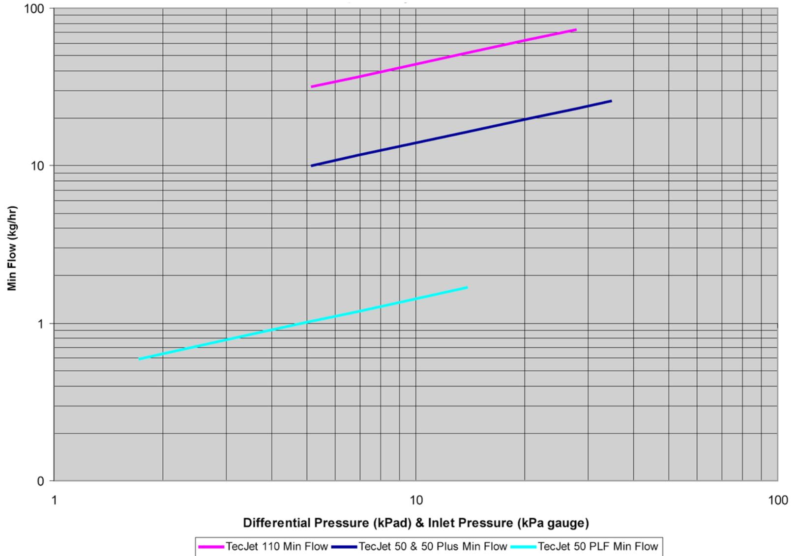
Figure 4-2. Minimum Specialty Gas Flow Capacity of TecJet 50 Plus, 50 Plus PF, 50, and 110 (Specialty Gas, SG=1, Sea Level)
