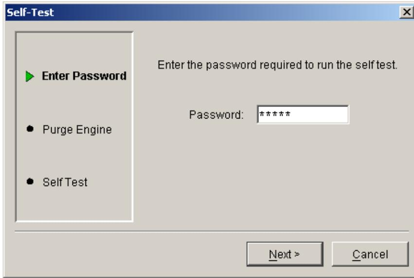
After the correct password is entered, you will be prompted to verify the engine is purged. **Be sure the fuel is shut-off and the engine is purged of any raw fuel.**
