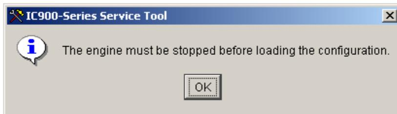
Once loading is completed, the new configuration settings take effect. Upon closing the Configuration File Editor screen, you will be prompted to save or not new or revised configuration settings to a file. This prompt does not appear if an already existing saved file was loaded.
