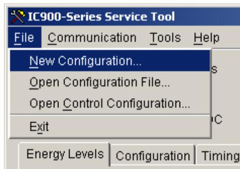
A Configuration File Editor opens with an incomplete configuration ready for edit to create a new IC-920/-922 configuration.
