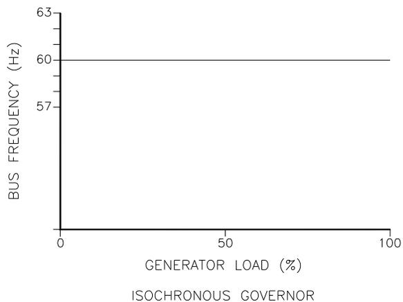
Figure 3-6. Isochronous Mode
