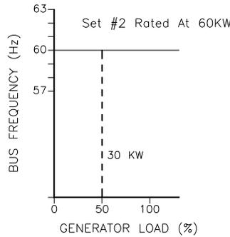
Isochronous Maintains Frequency and Load Swings
