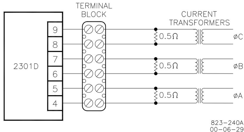
Figure 5-1. Temporary Wiring for Transformer Phase Correction
