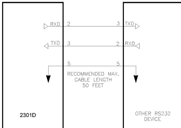
Figure 2-3. RS-232 Pin assignments for Serial Communication Cable
