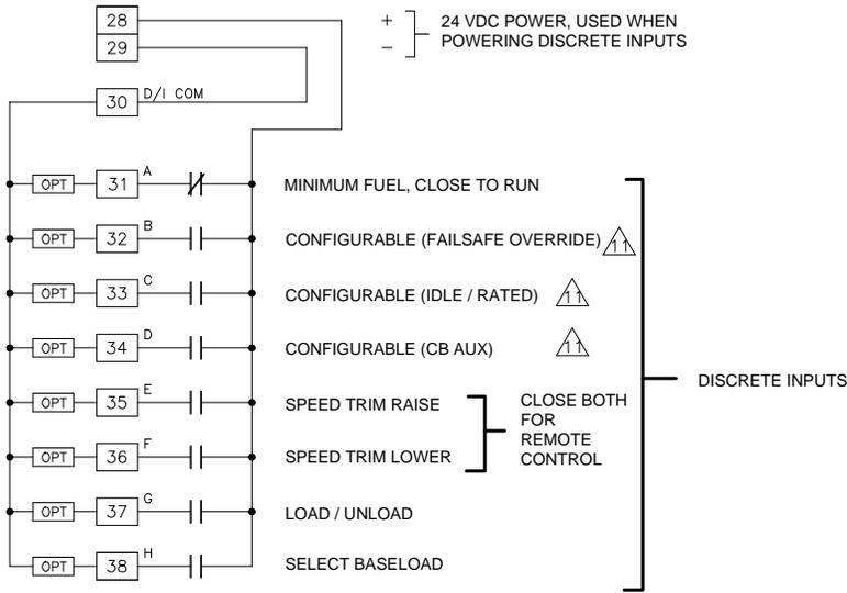
DISCRETE INPUTS WITH EXTERNAL POWER SUPPLY
