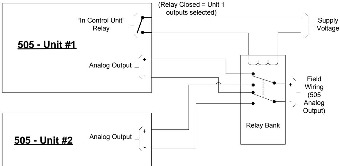
Figure 2-15n. Analog Output Switching Diagram
