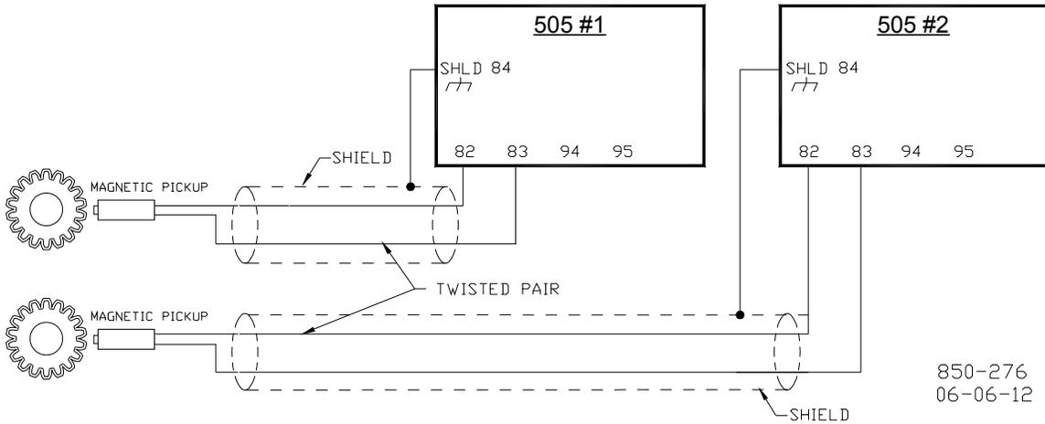
Figure 2-15c. Optional Speed MPU Input Diagram – Different Probes
