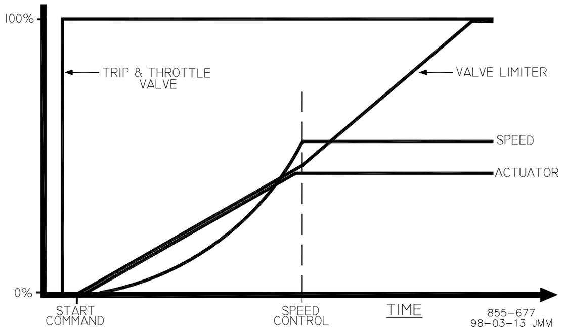
Figure 3-3. Automatic Start Mode Example
