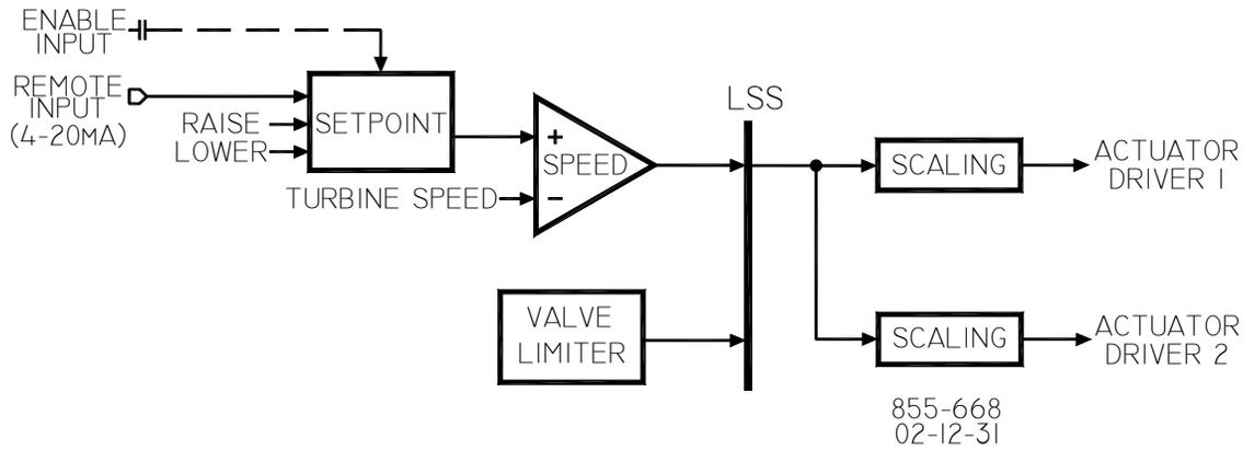
Figure 1-4. Single or Split-Range Turbine Configurations
