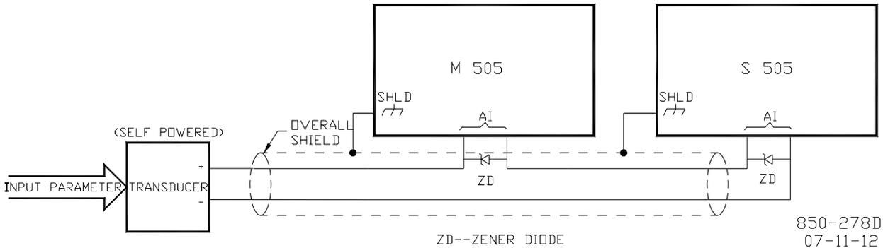
Figure 2-15j. One Transducer Driving Both 505 Inputs
