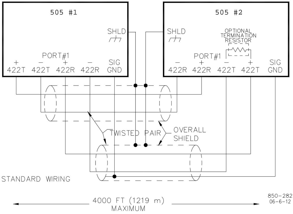
Figure 2-15q. Typical RS-422 Communications Between Master and Slave
