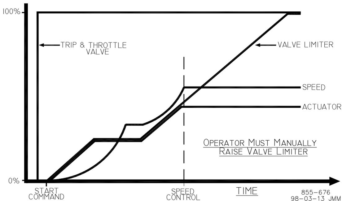
Figure 3-2. Semiautomatic Start mode Example
