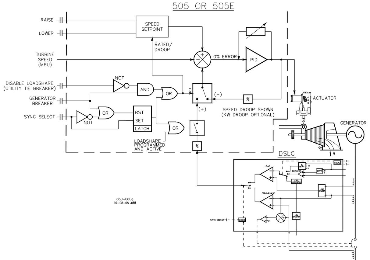
Figure 3-10. Load Sharing Logic
