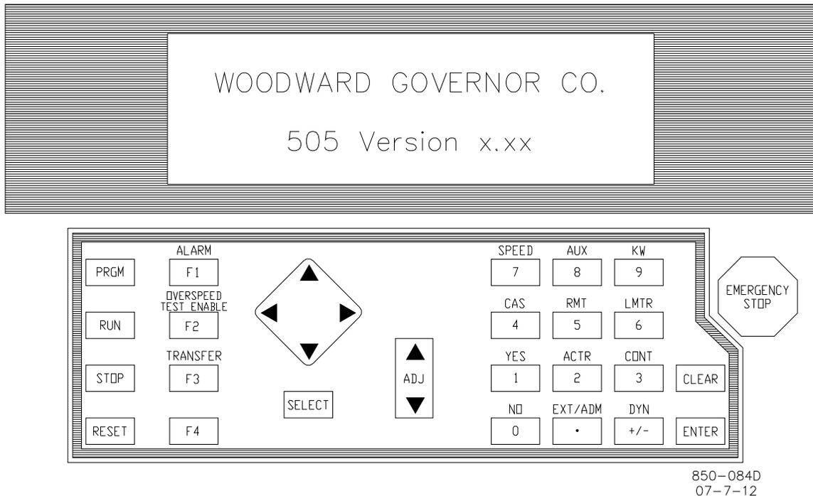
Figure 5-3. 505 Keypad and Display
