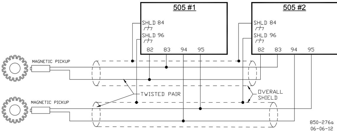
Figure 2-15d. Recommended Speed MPU Input Diagram – Common Probes
