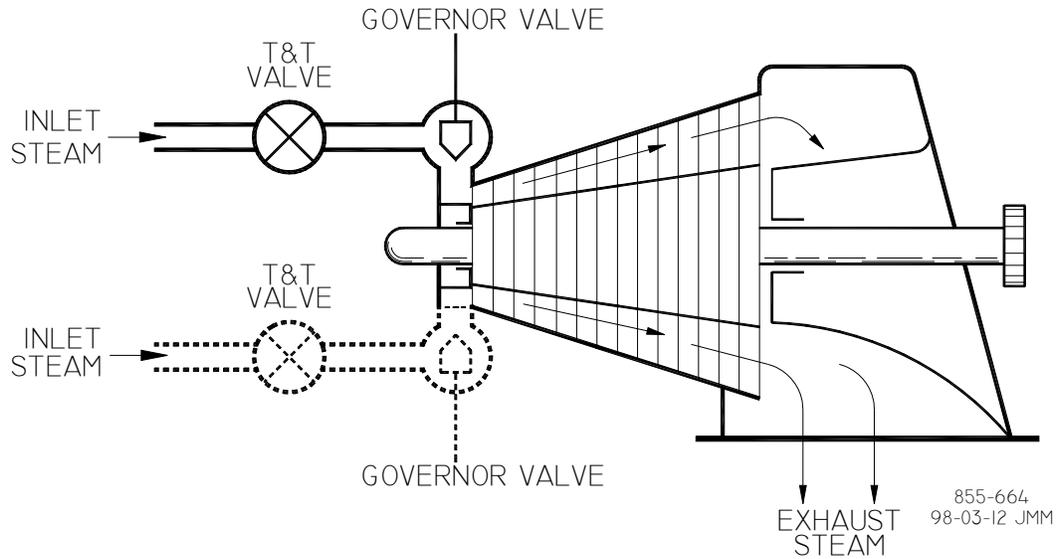
Figure 1-1. Typical Single or Dual Inlet Steam Turbine
