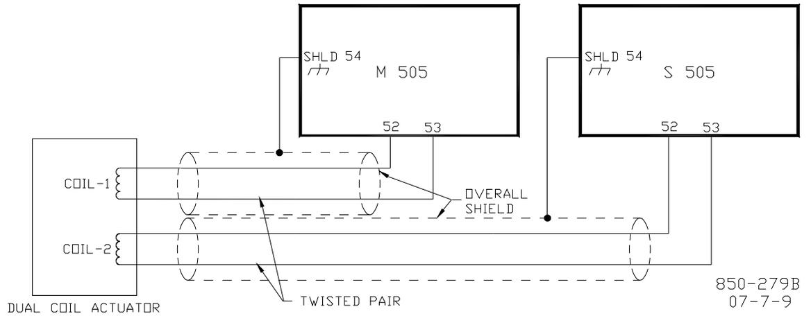
Figure 2-15l. Dual Coil Applications
