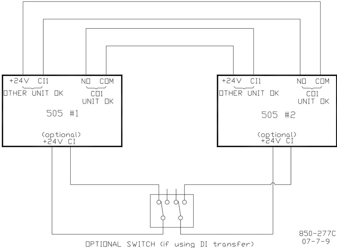
Figure 2-15g. Redundant Contact Input Diagram – DPDT Switches
