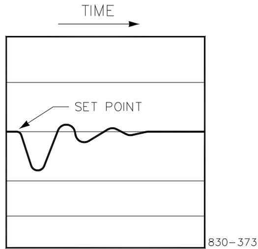
Figure 5-19. Typical Response to Load Change
