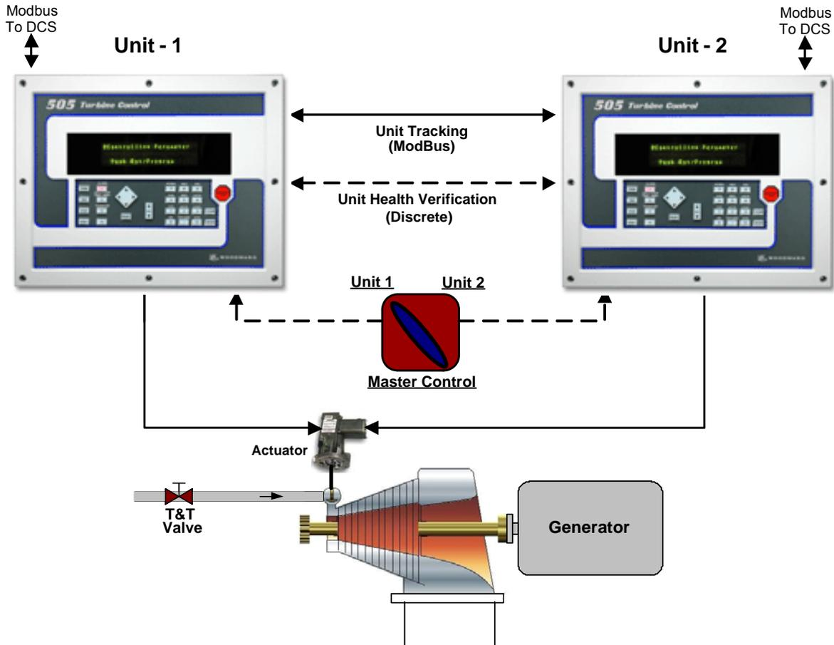
Figure 3-14. Redundant 505 Configuration Diagram
