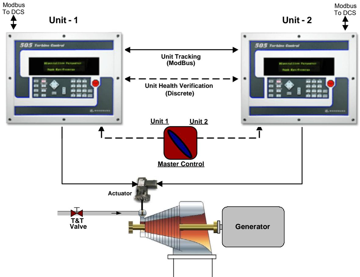
Figure 1-7. Typical Redundant 505 Application Configuration
