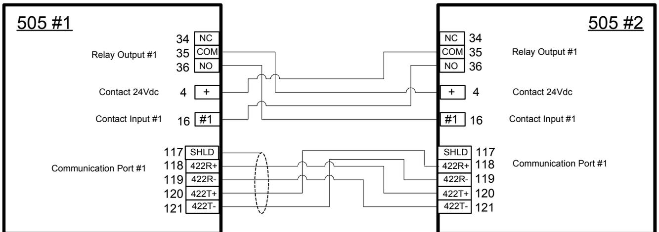
Figure 2-15a. Redundant Interface Connections
