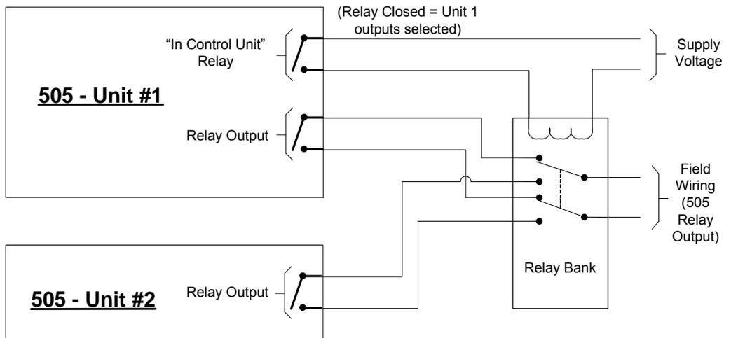
Figure 2-15p. Relay Output Switching Diagram
