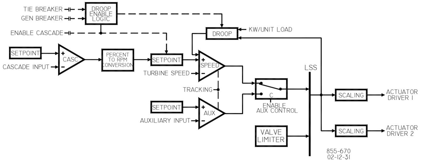
Figure 1-6. Single or Split-Range Turbine Configurations
