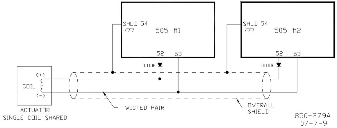
Figure 2-15k. Single Shared Coil Applications
