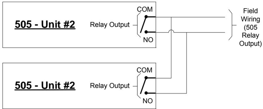
Figure 2-15o. Relay Outputs (positive logic)
