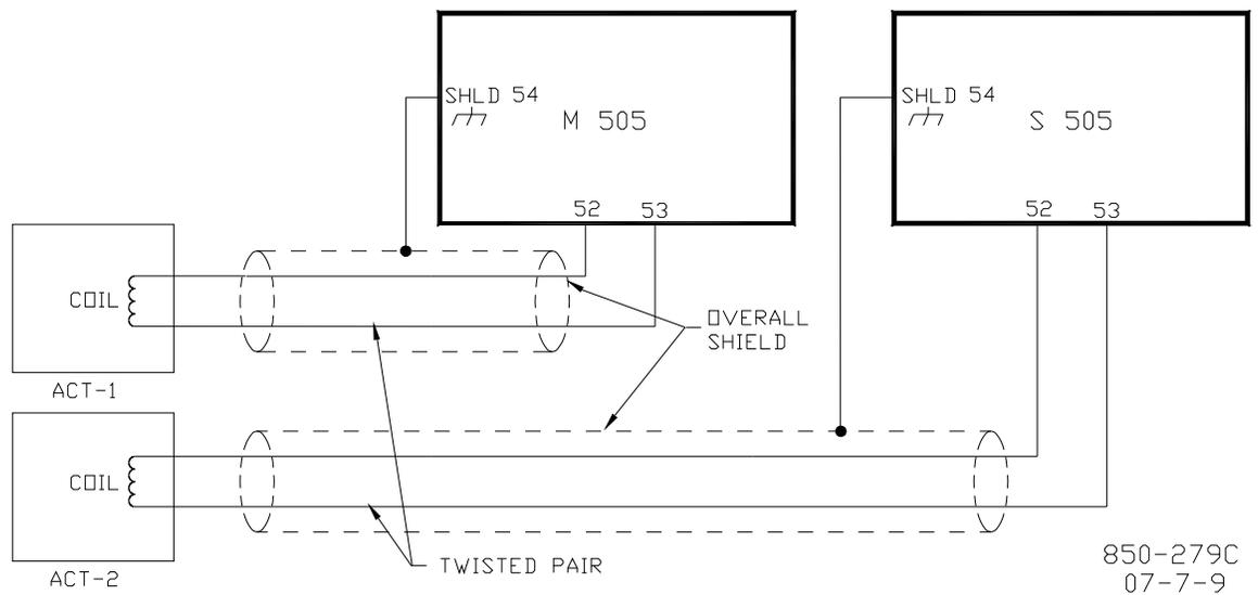
Figure 2-15m. Parallel Actuator Applications
