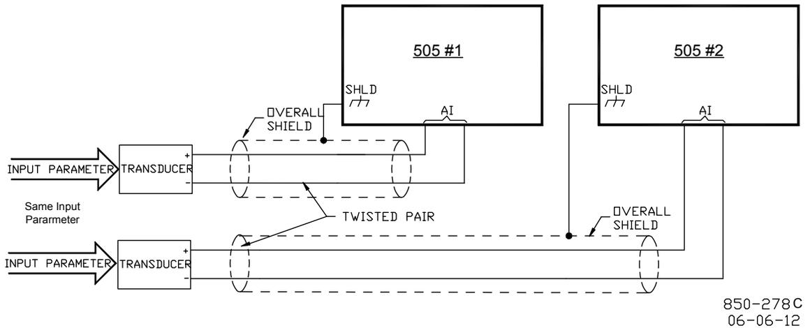
Figure 2-15h. Two Transducers with One Transducer for each 505 Unit
