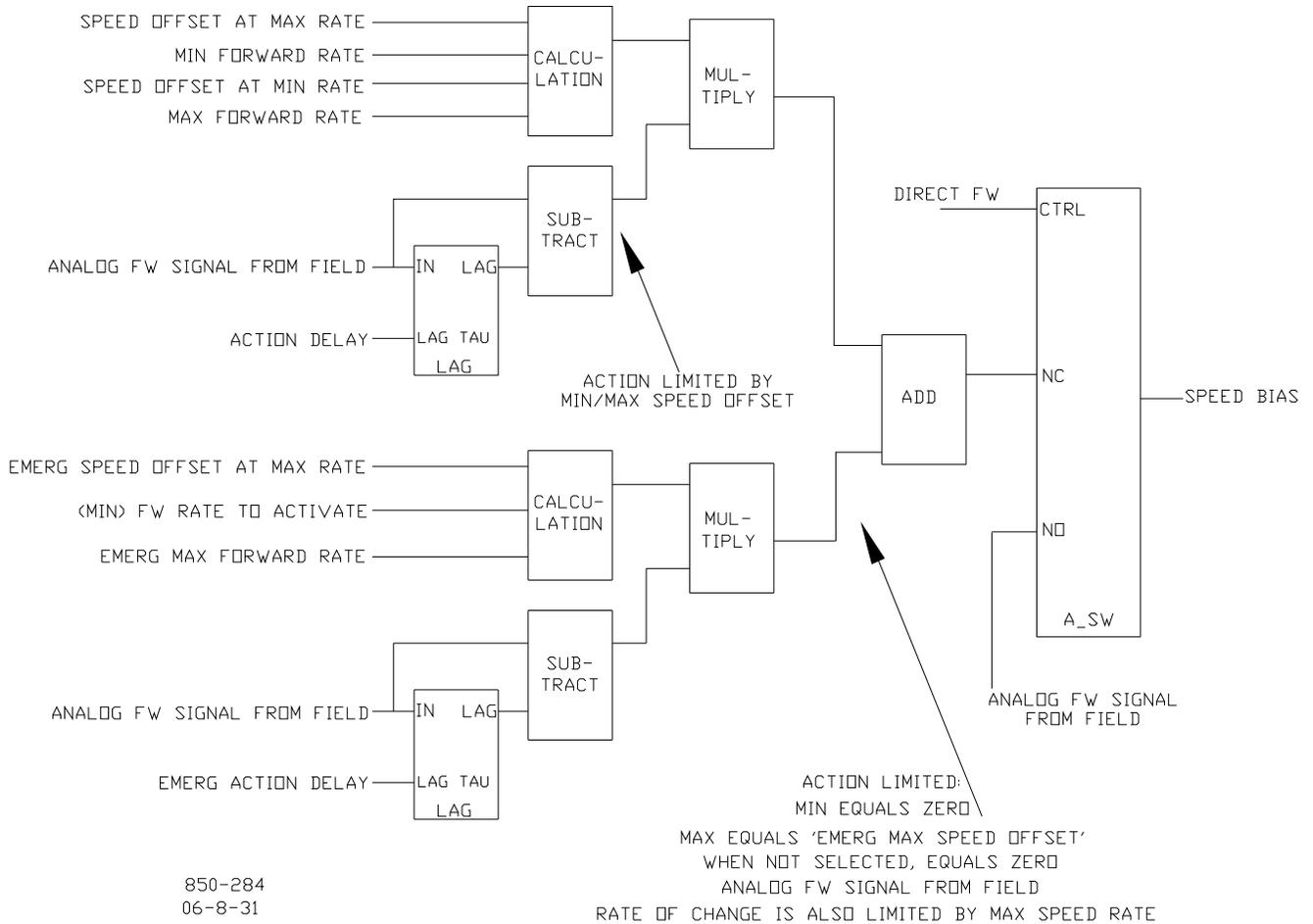
Figure 3-11. Typical Anti-surge Valve and Speed Feed-Forward Logic Trend
