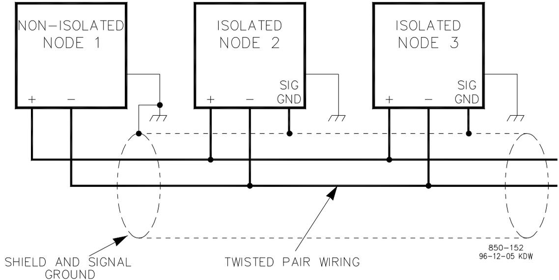
Figure 2-14. Alternate Multipoint Wiring without a Separate Signal Ground Wire
