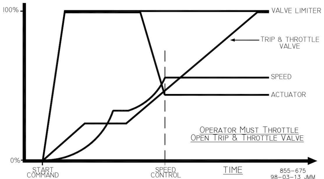
Figure 3-1. Manual Start Mode Example
