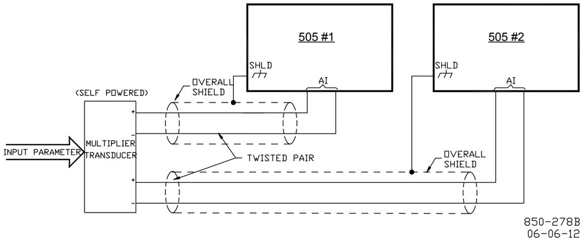
Figure 2-15i. One Transducer Using a Current Splitting/Isolation Device
