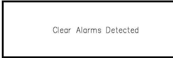
3. To go from the Clear Alarms Detected header to the Top Level/Root display, press the CLEAR key.
