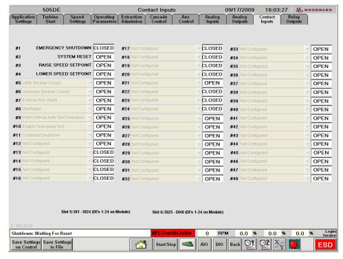
Figure 3-27. Contact Inputs Screen
