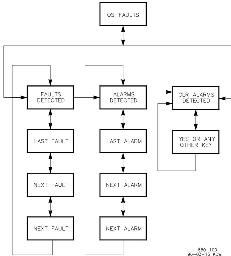
Figure 7-1. OPSYS\_Faults Display Sequence
