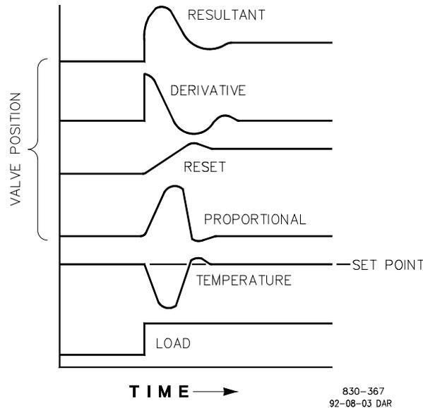
Figure 8-7. Closed Loop Proportional, Integral and Derivative Action
