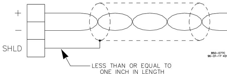
Figure 3-9. Shielded Wire Connections
