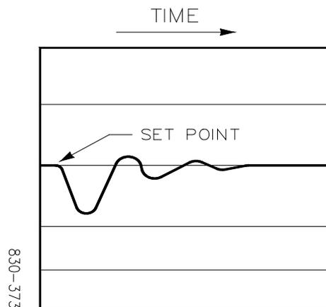
Figure 8-8. Typical Response to Load Change
