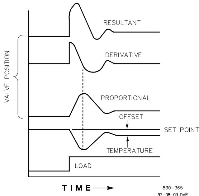
Figure 8-5. Closed Loop Proportional and Derivative Action
