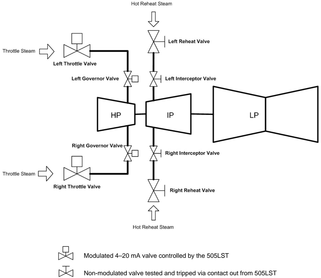
Figure 1-1. Turbine Type 1 Schematic
