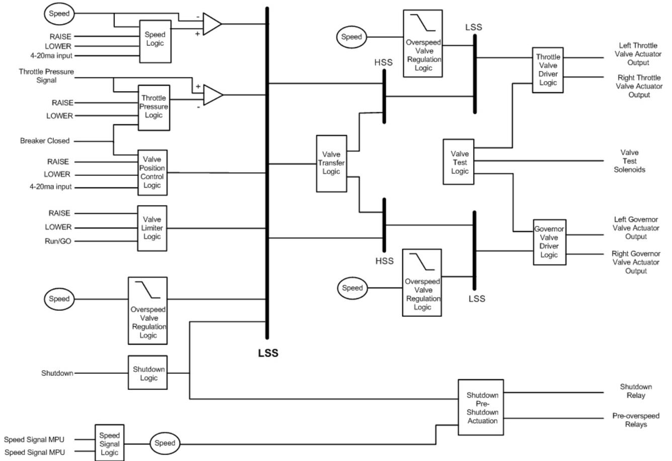
Figure 1-3. Turbine Type 1 Block Diagram
