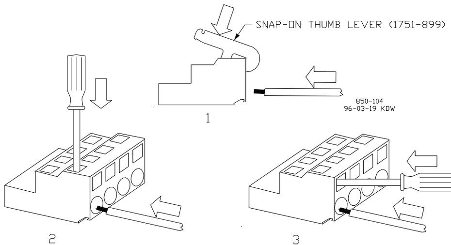
Figure 3-5. CageClamp Terminal Blocks
