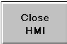
In the lower right corner of the Main Menu screen, the Close HMI button will terminate the HMI/CCT application but has no effect on the 505CC-2 or its controlling of the turbine/compressor unit.
