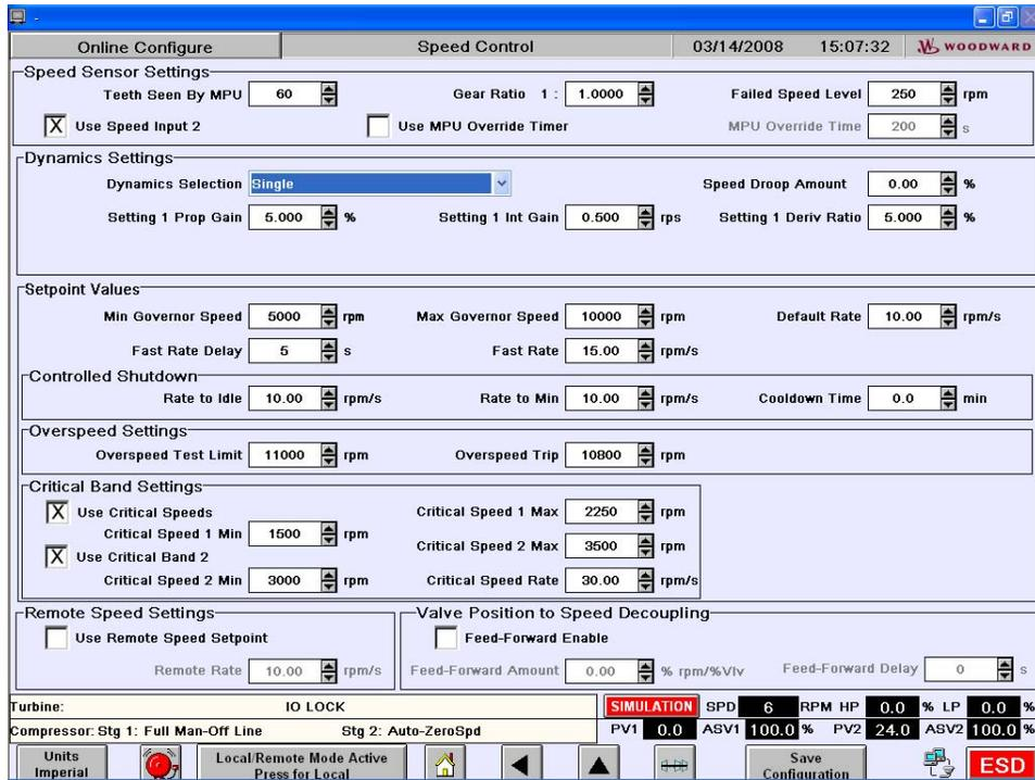
Figure 4-4. Turbine Speed Control Configuration Screen
