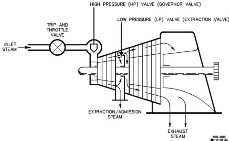
Figure 2-4. Typical Extraction or Extraction/Admission Steam Turbine
