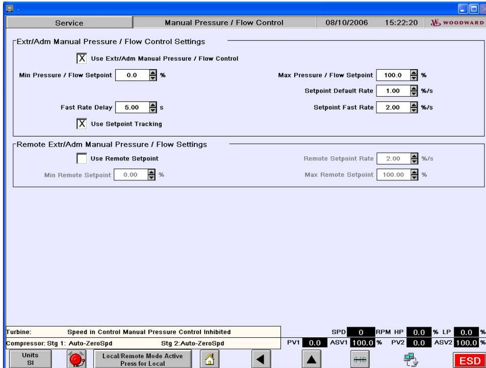
Figure 4-7. Turbine Extr/Adm Manual Pressure (Flow) Configuration Screen
