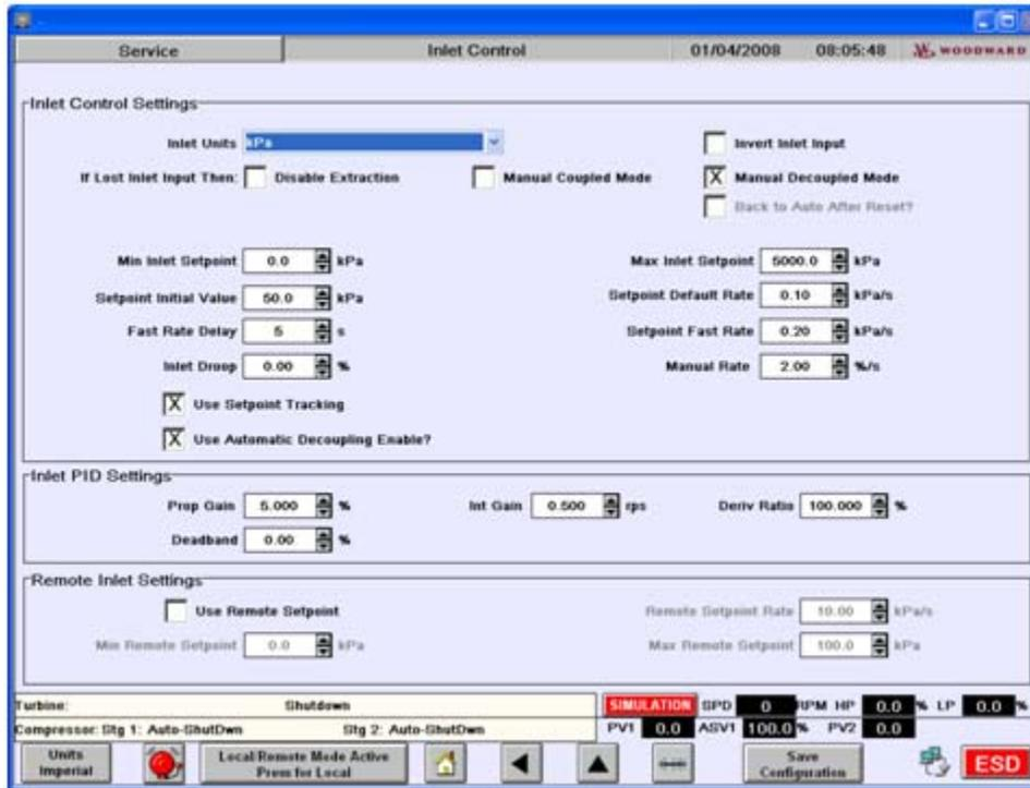
Figure 4-13. Turbine Inlet/Exhaust Control Configuration Screen
