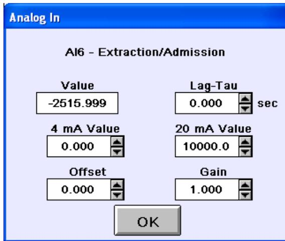
Figure 4-17. Analog Input Calibration Pop-Up
