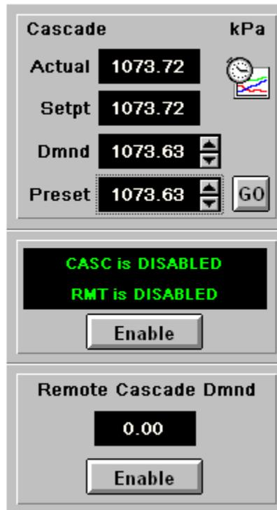
Figure 5-9. Turbine Run Screen Cascade Controller
