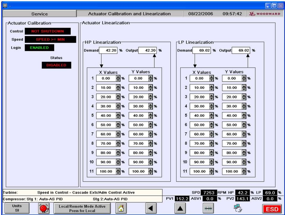
Figure 5-16. Turbine Actuator Cal/Linearization Screen
