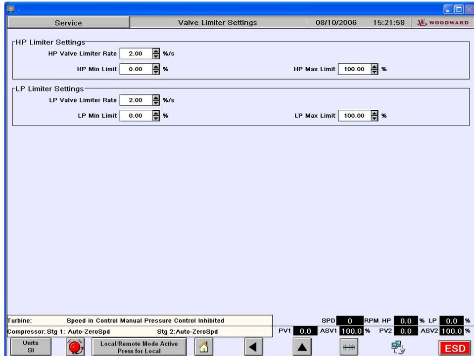
Figure 4-6. Turbine Valve Limiter Configuration Screen
