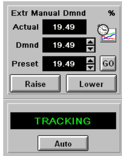
Figure 5-11. Turbine Run Screen Manual Pressure/Flow Demand
