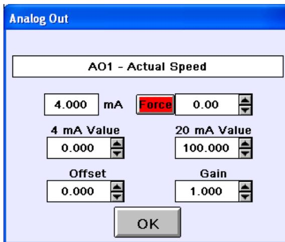
Figure 4-18. Analog Output Calibration Pop-Up
