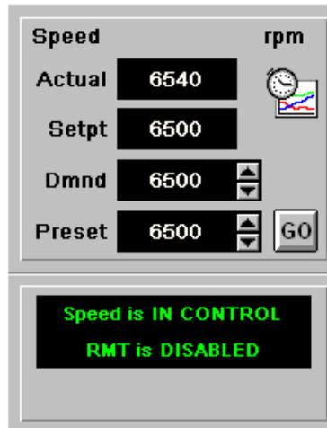
Figure 5-8. Turbine Run Screen Speed Controller
