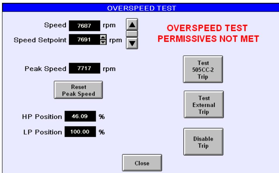
Figure 5-6. Turbine Overspeed Test Pop-Up
