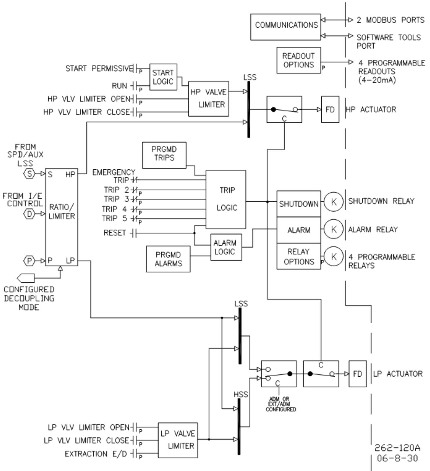
Figure 2-3. Overview of 505CC-2 Turbine Control Functionality
