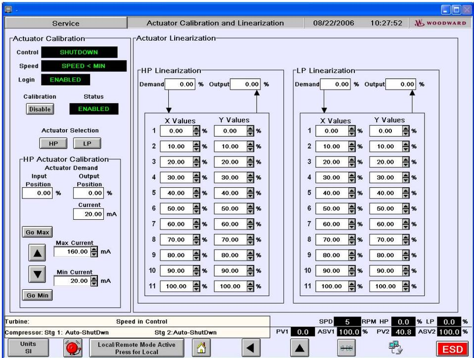
Figure 5-17. Turbine Actuator Cal/Linearization Screen
