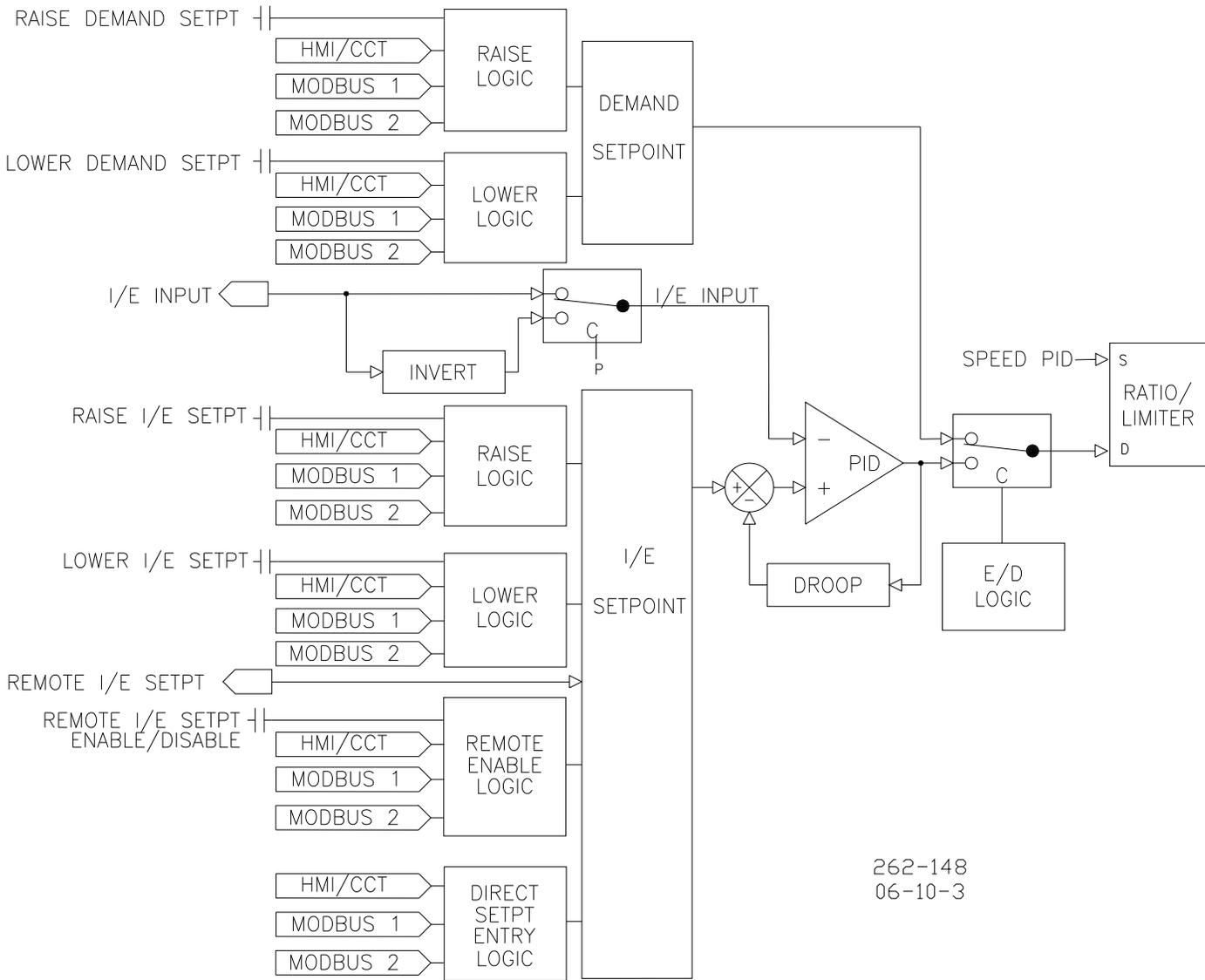
Figure 2-9. Inlet/Exhaust Decoupling Control Functional Diagram
