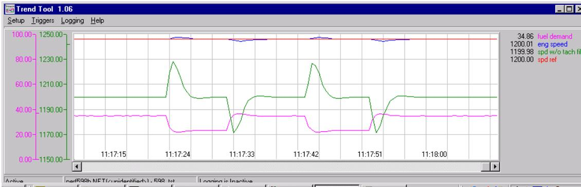
21. This trace shows results of just increasing Gain from 1.235 to 3.0. Gain Ratio and Window Width remain disabled. Peak rpm is reduced approximately 10–12 rpm.
