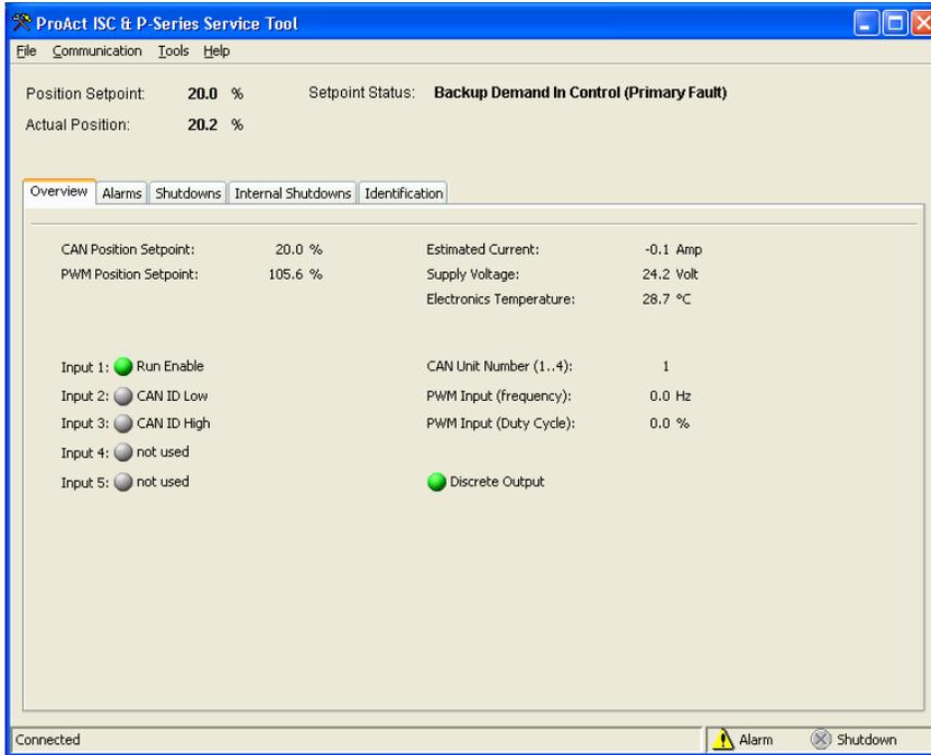
Figure 4-2. Example Service Tool Screen
