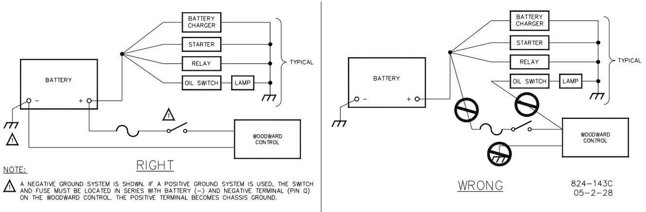
Figure 2-3. Correct and Incorrect Wiring to Power Supply
