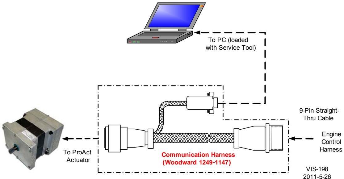
Figure 4-1. Communication Harness Connections
