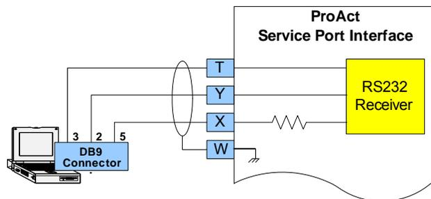
Figure 4-3. Typical Programming Datalink Harness Wiring
