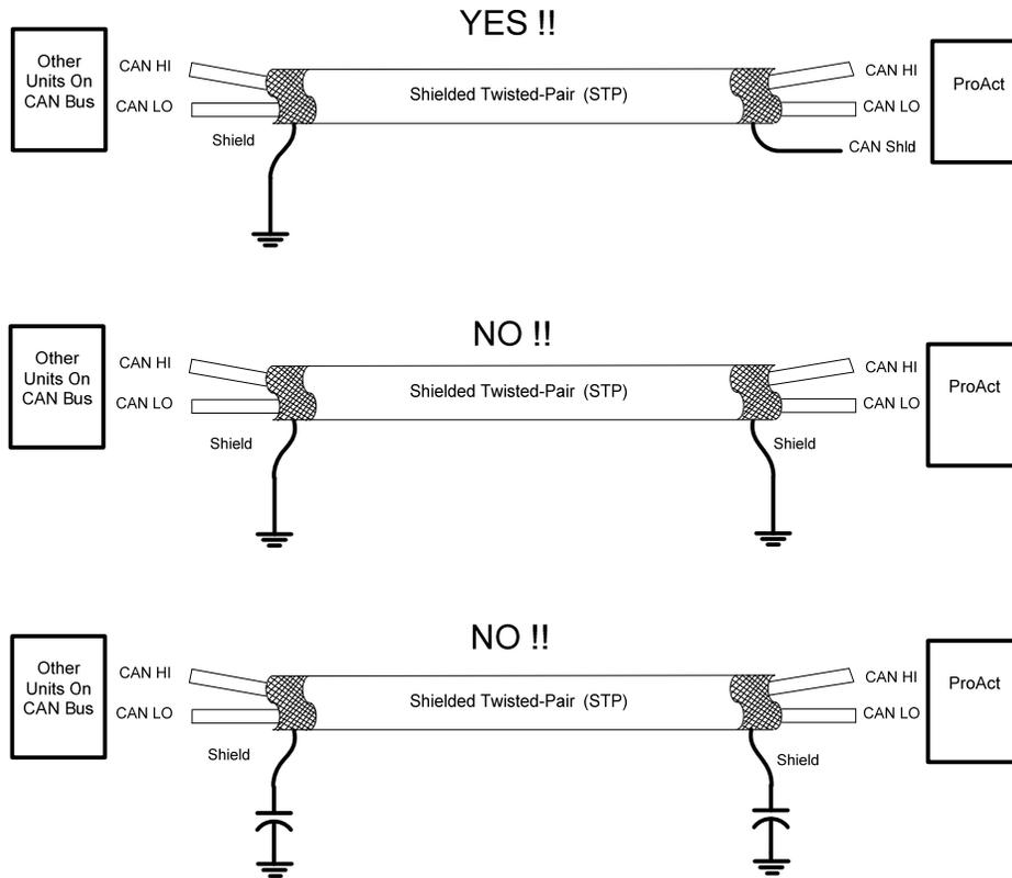
Figure 2-4. CAN Shielding
