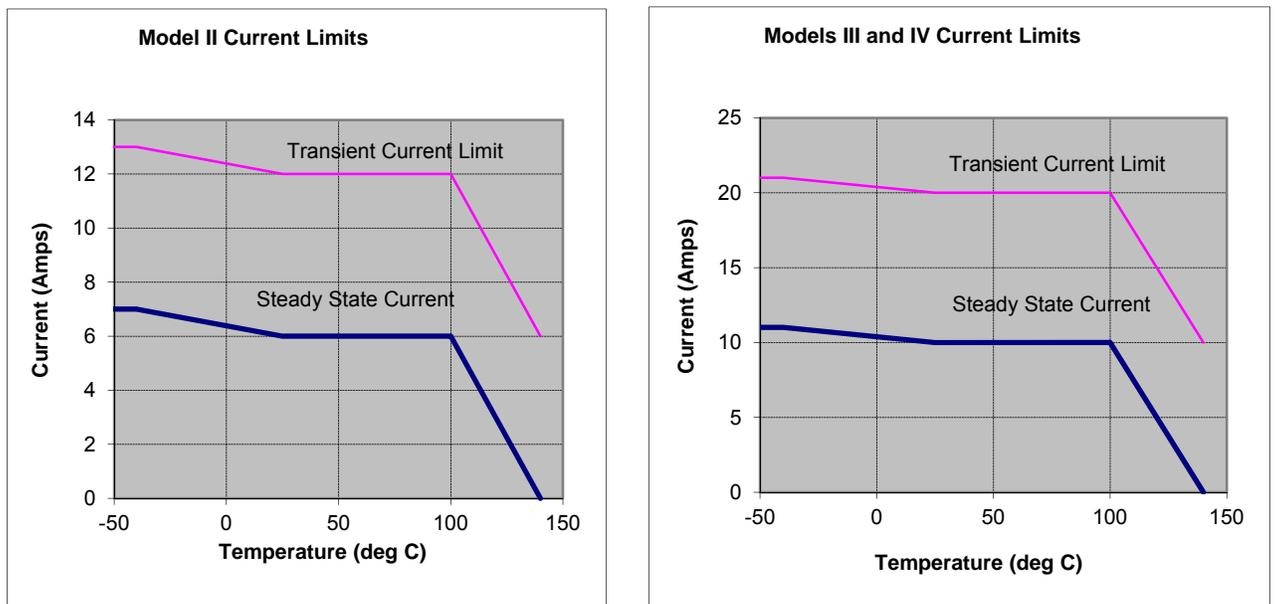
Figure 3-4. Example Temperature vs. Current Limit Curves
