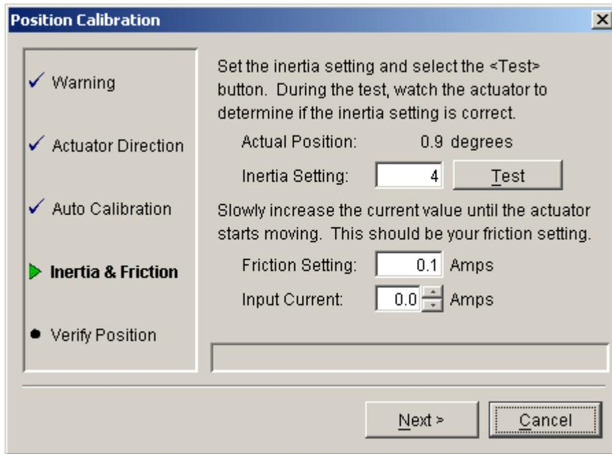
Figure 6-3. Auto Cal Inertia &amp; Friction Screen
