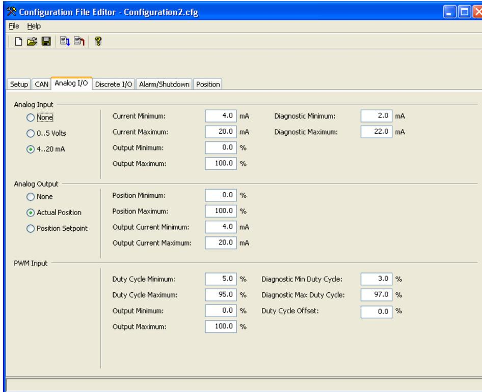
Figure 5-3. Configuration Editor—Analog I/O Tab
