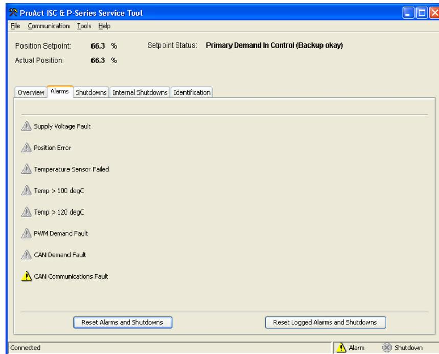
Figure 4-5. Service Tool—Alarms Tab
