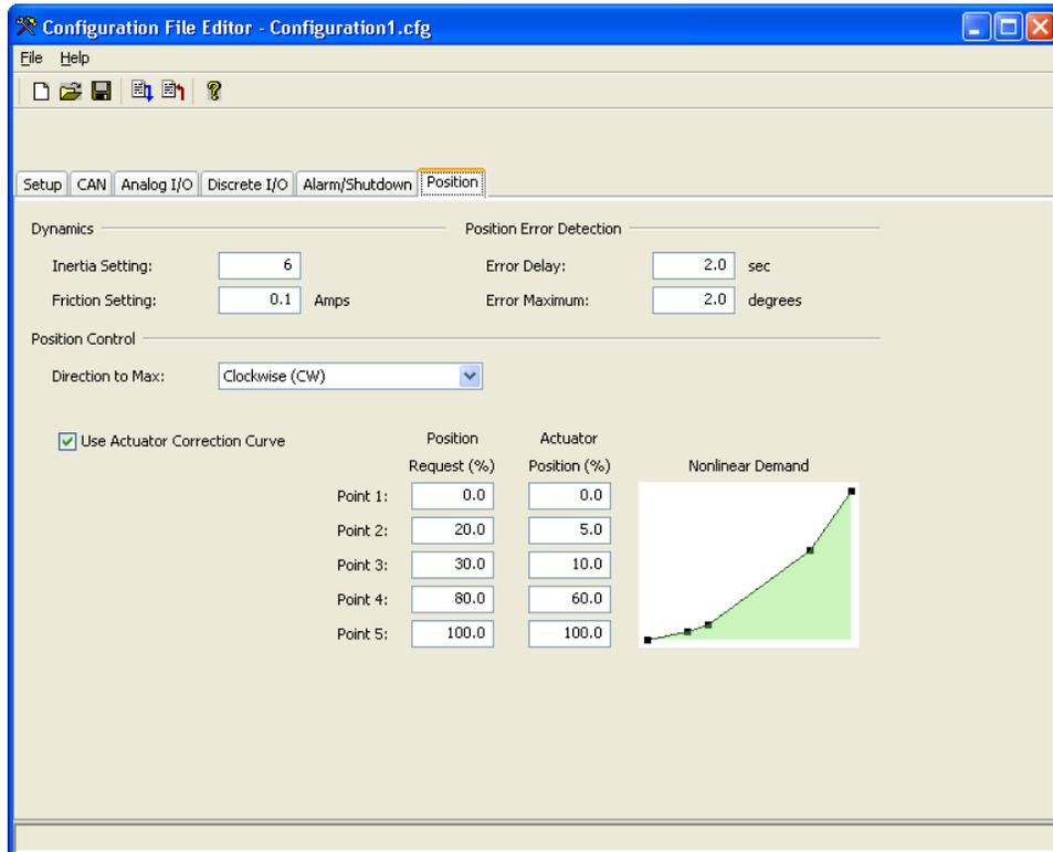
Figure 5-6. Configuration Editor—Position Tab
