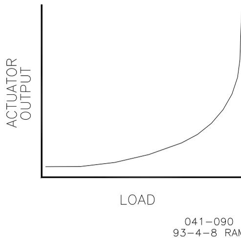
Figure 4-6. Non-linear Valve Power Curve
