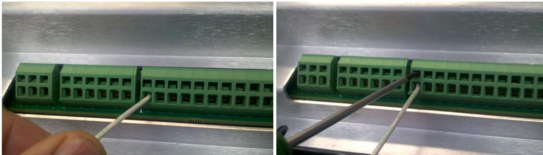
Figure 2-1. Installation of Wiring into Terminal
