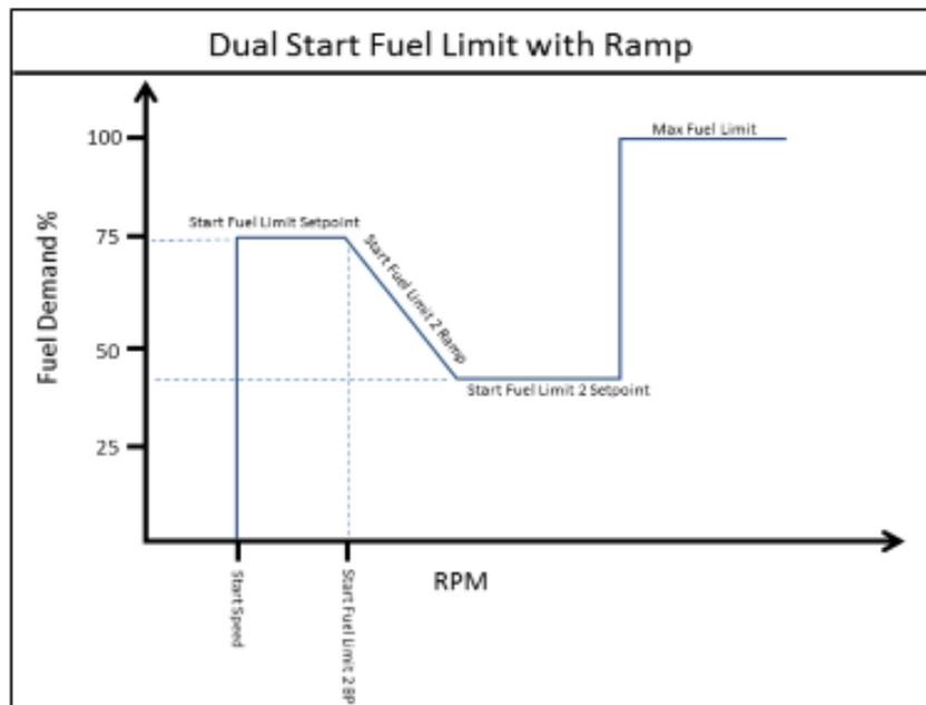
Figure 3-3. Dual Start Limit Function
