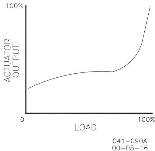
Figure 4-7. Non-linear Valve Power Curve for Turbocharged Engine
