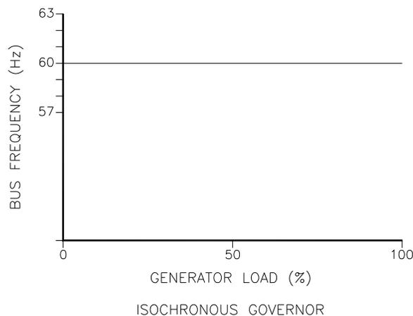
Figure 3-6. Isochronous Mode
