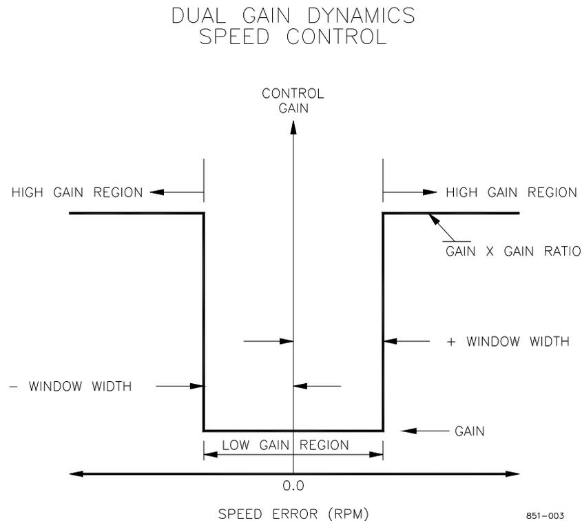
Figure 4-2. Control Gain as a Function of Speed Error
