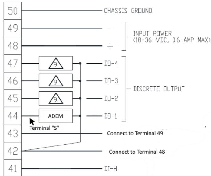
2.0 In the 2301E Configuration Mode, select the Actuator Output Type to 4. This activates Discrete Output #1 for a PWM output.
