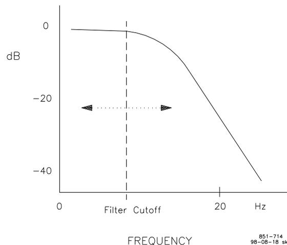
Figure 4-4. Speed Filter
