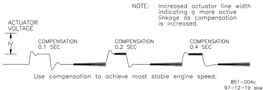
Figure 4-5. Typical Transient Response Curves
