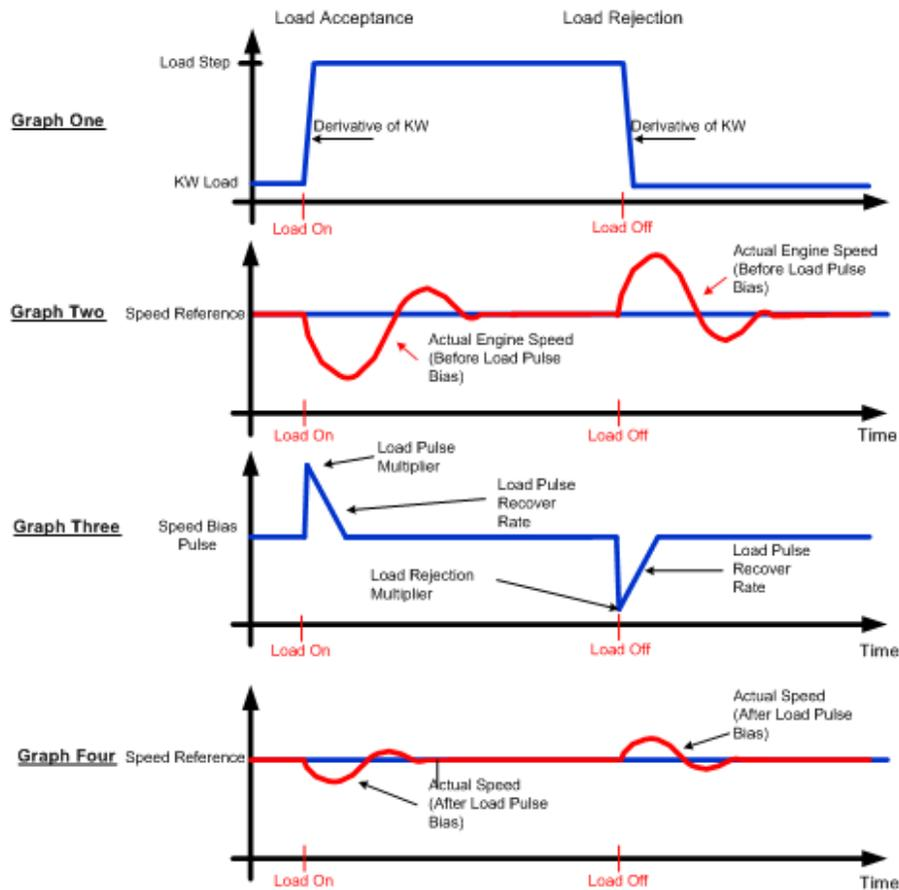
Figure 3-9. Load Pulse / Rejection
