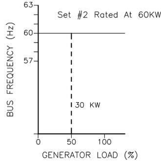
Isochronous Maintains Frequency and Load Swings
