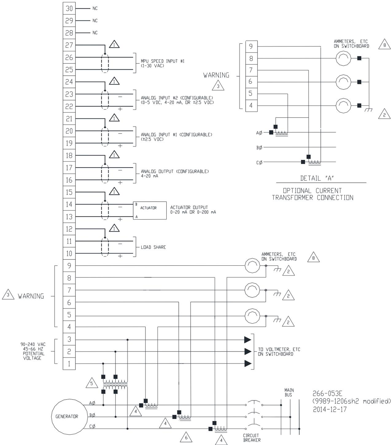
Figure 1-2a. 2301E Control Wiring Diagram (sheet 1)
