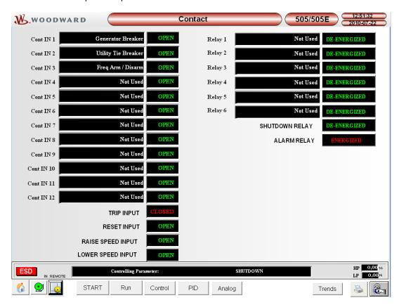
The configuration and status of the twelve configurable contact inputs is displayed on the left side of the screen. A CLOSED indication means that input of the 505 control is being held high or a logic 1. An OPEN indication means the input is being held low or a logic 0.
