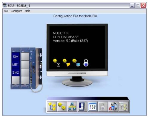
The bottom of the SCU window contains a toolbox that includes all the tools you need to use the SCU.
