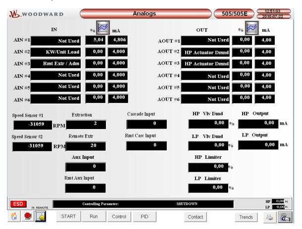
Analog inputs are displayed in the engineering units, based on the 505 configuration. Turbine speed and speed setpoint value are displayed. The actuator(s) output is displayed in mA. The valve demand and limiter position is displayed on this screen.
