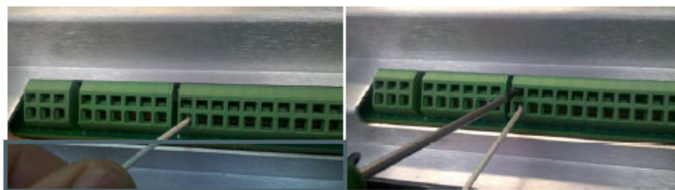
Figure 2-3. Installation of Wiring into Terminal
