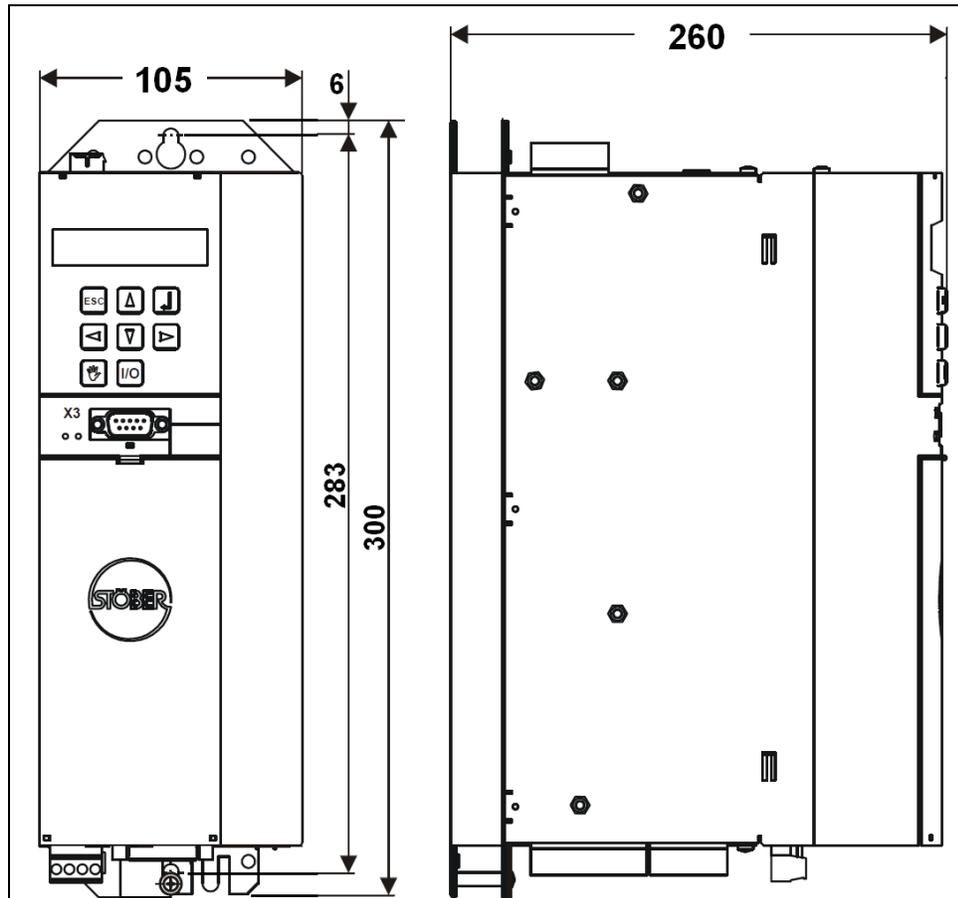
Figure 5-1. EM-80/300 Driver Dimensions (mm)
