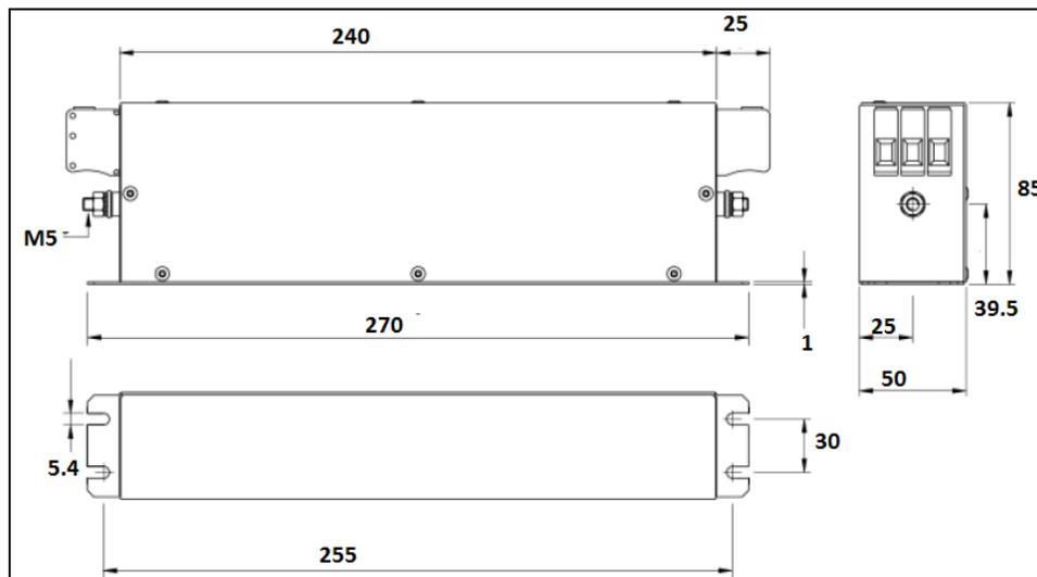
Figure 5-5. 1326-1125 Filter Assembly (mm)
