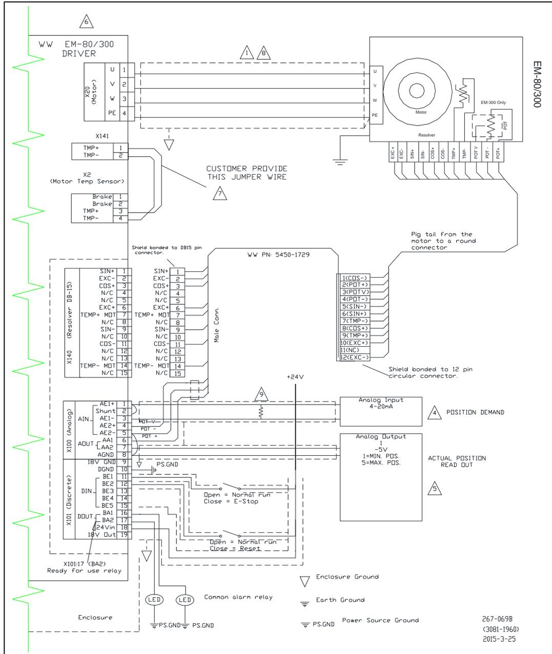
Figure 3-2b. Control Wiring Diagram (right half)
