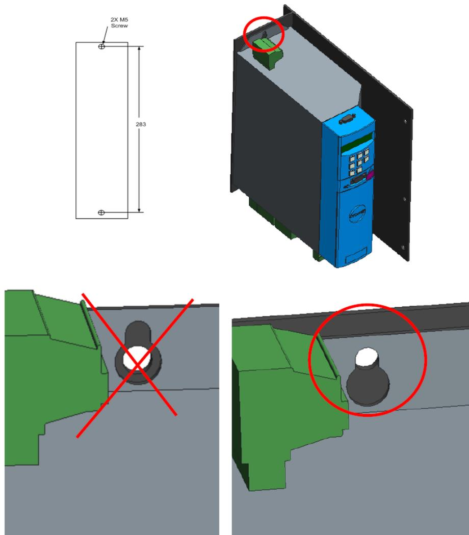
Figure 5-3. Driver Mounting Profile Dimension
