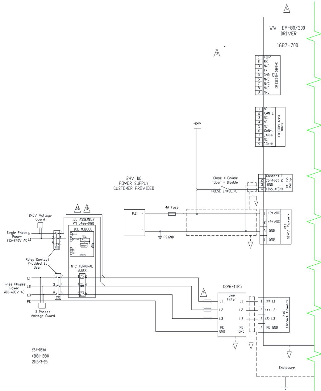
Figure 3-2a. Control Wiring Diagram (left half)
