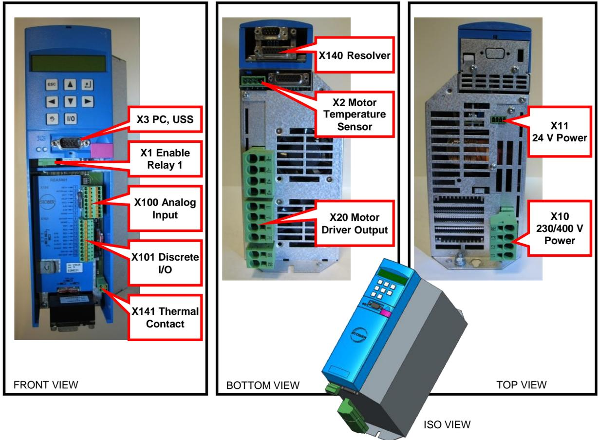
Figure 5-4. Driver Electrical Connection
