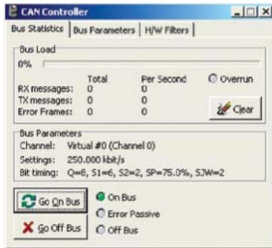
If there is traffic on the bus, the “Bus Load” bar will give you an idea of how much bandwidth is being consumed. If the “Error Passive” indicator illuminates, there are 3 possible reasons:
