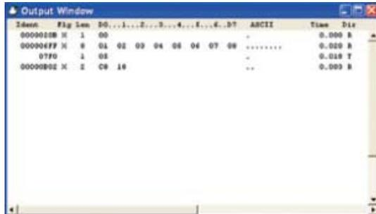
9. In CanKing, transmit a message on address \$7f0 with any data.
