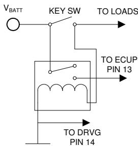
E-Stop switches are placed between the NO contact and pin 13 of the module. The XDRG is the transducer ground return.
