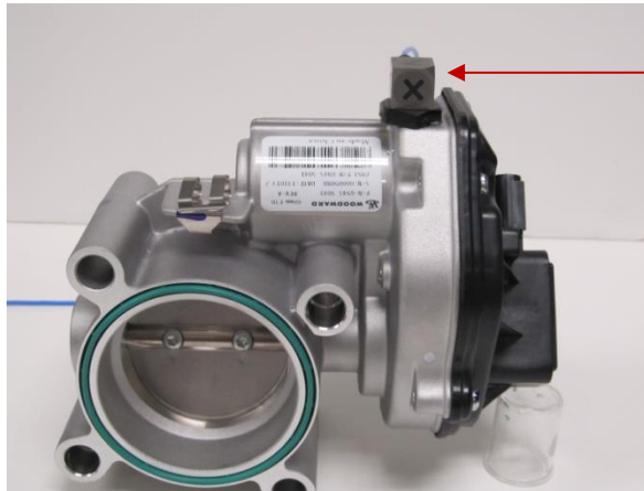
Additional Vibration Sensor Location #1
