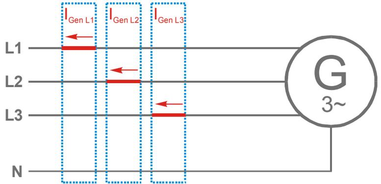
Figure 3-24: Monitoring - calculated generator ground fault
