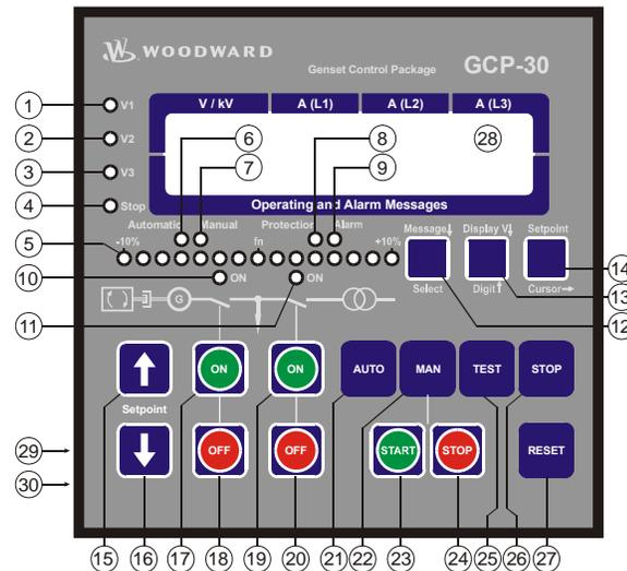
Figure 2-2: Front panel GCP-32
