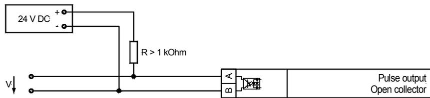
Figure 3-9: Pulse output
