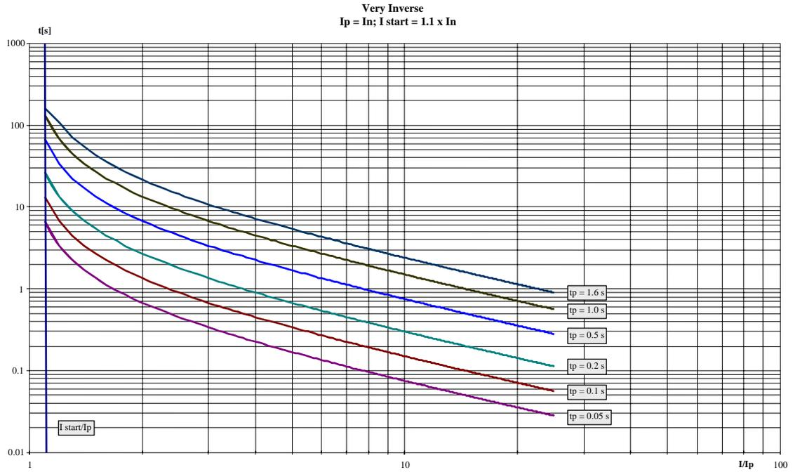
Figure 6-3: Inverse time-overcurrent - characteristic "very inverse"
