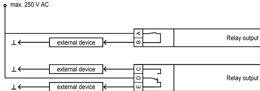
Figure 3-8: Relay outputs
