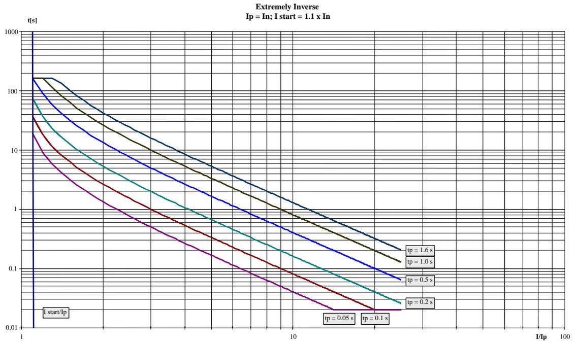
Figure 6-4: Inverse time-overcurrent - characteristic "extremely inverse"
