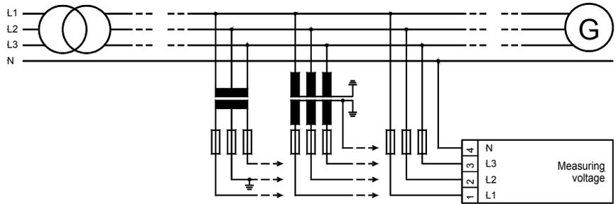
Figure 3-4: Measuring inputs - voltages
