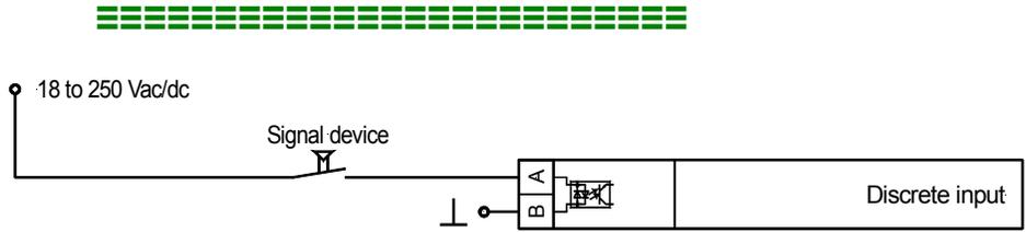
Figure 3-7: Discrete inputs
