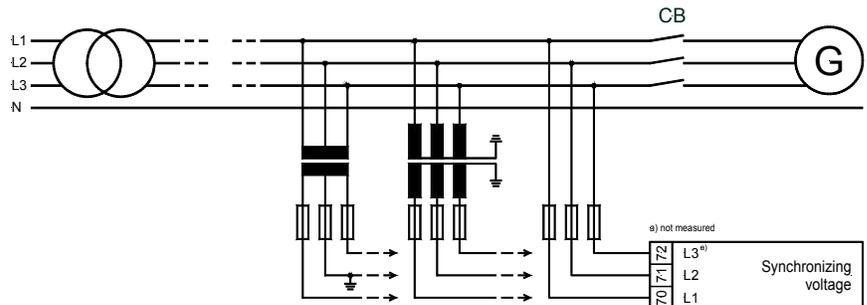
Figure 3-5: Measuring inputs - synchronizing voltage
