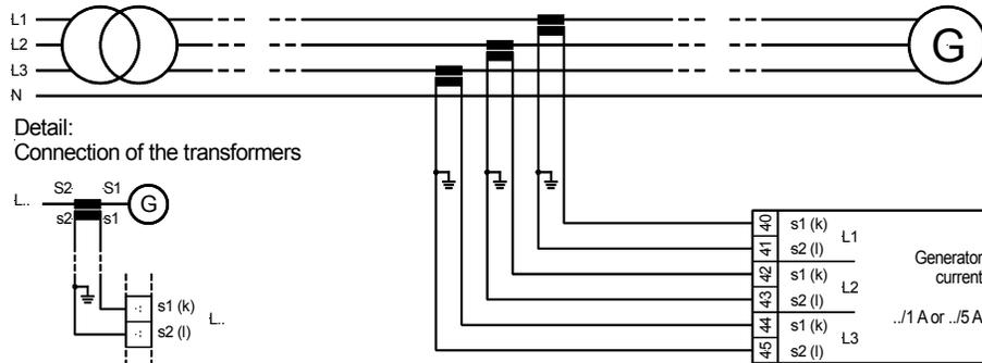
Figure 3-6: Measuring inputs - current
