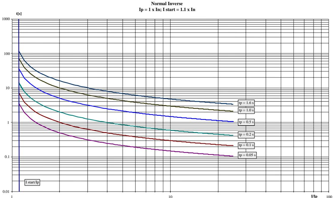
Figure 6-2: Inverse time-overcurrent - characteristic "normal inverse"
