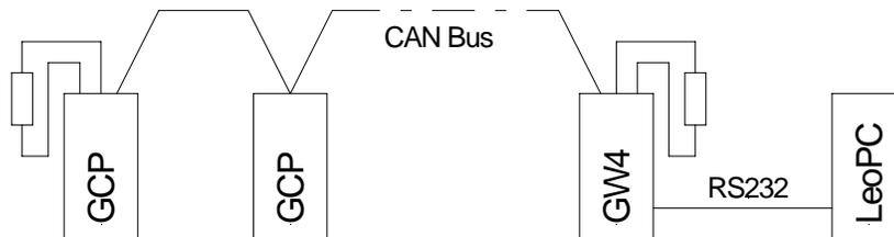
Observe the notes about termination (termination resistor) of the CAN bus under Connection on page 5. Up to 4 GCPs can be connected to a GW 4.
