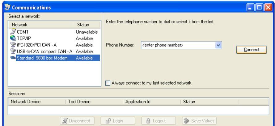
Figure 4-36: Connecting ToolKit with a landline modem
