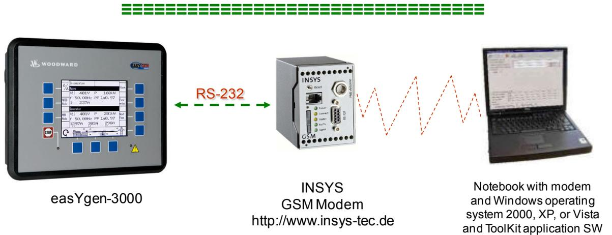
Figure 4-28: Connecting a GSM modem
