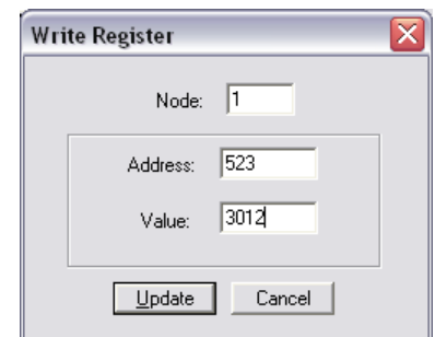
Figure 3-33: Modbus - write register - acknowledge alarm message
