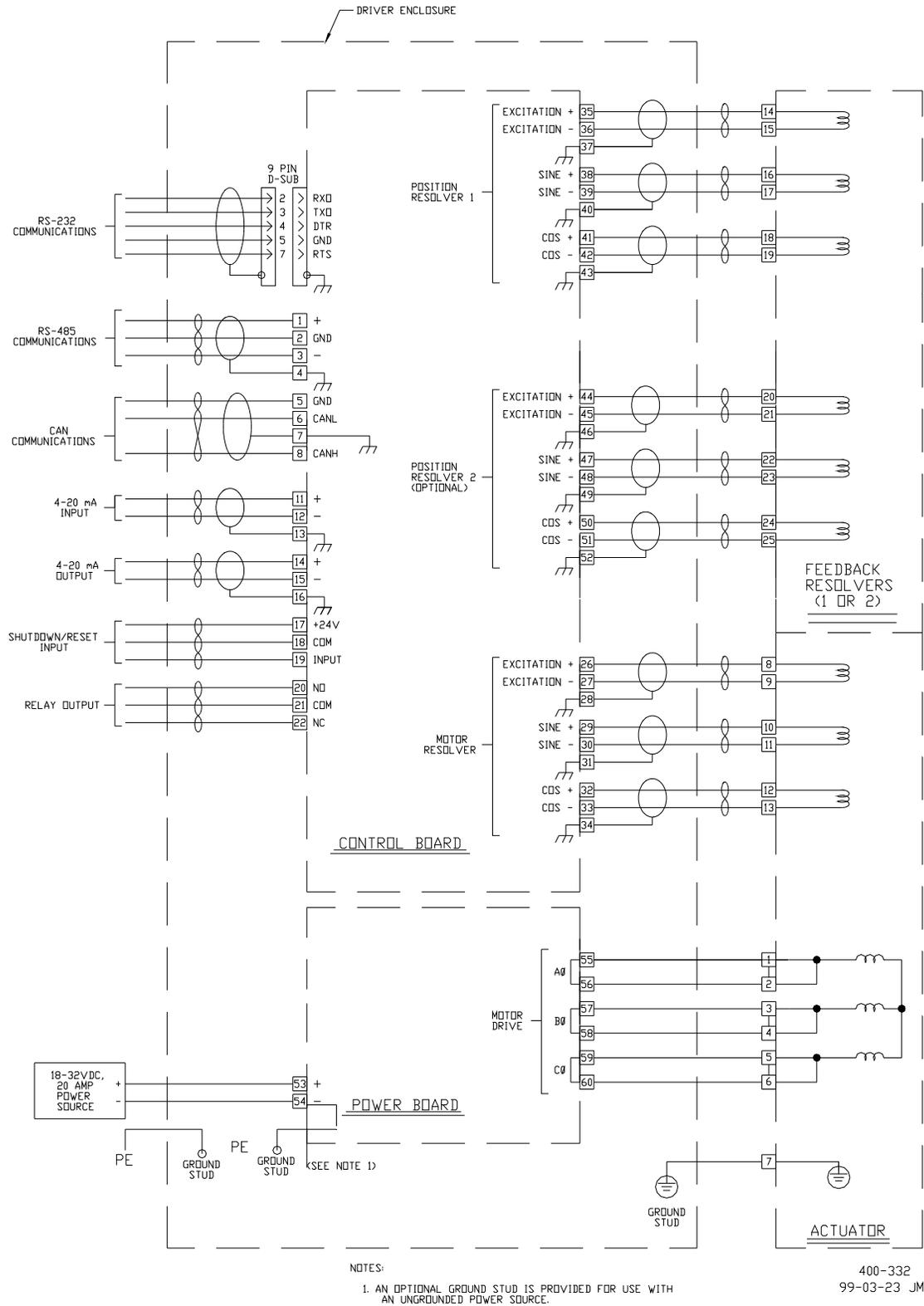
Figure 2-2a. Wiring Diagram (EM Driver Connections Shown)
