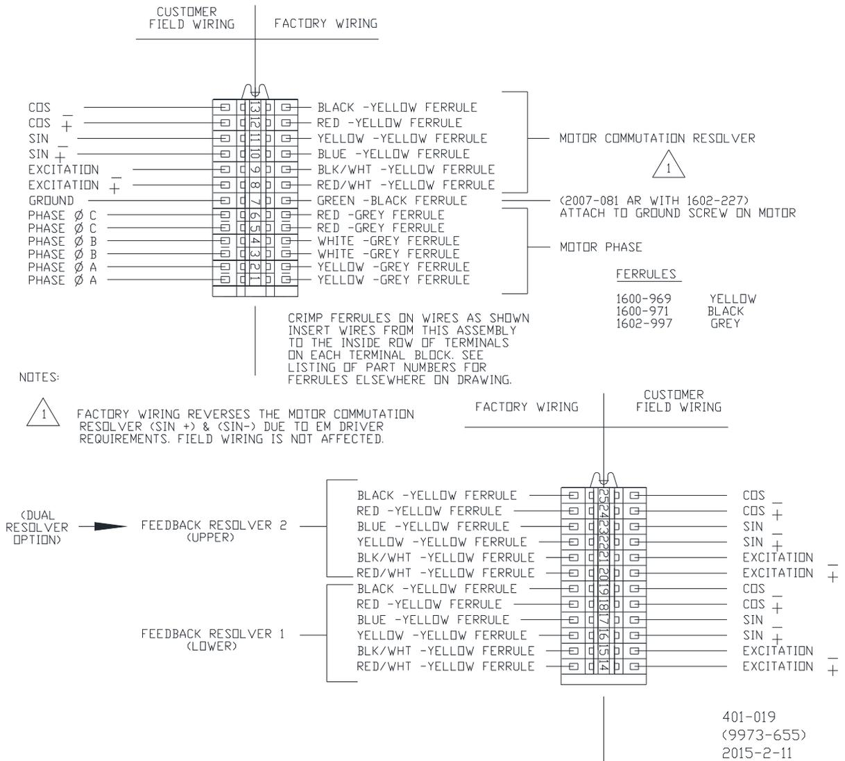
Figure 2-2b. Wiring Diagram (EM Driver Connections Shown)
