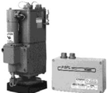
The **PGPL Actuator/Driver** is a drop-in replacement for PG-PL mechanical governors, and is an electro-hydraulic actuator with a proportional driver interface which can be used with electronic controls providing a 0 to 200 mA position signal. The actuator is designed for use with Woodward controls.
