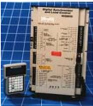
The **DSLCTM** control is a microprocessor-based synchronizer and load control designed for use on three-phase ac generators equipped with Woodward or other compatible speed controls and compatible automatic voltage regulators. The DSLC control is a synchronizer, a load sensor, a load control, a dead bus closing system, and optionally a VAR/PF and process control, all integrated into one powerful, yet convenient package.
