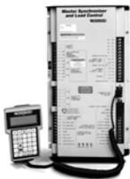
The **MSLC** control is a microprocessor-based load control designed for three-phase electric power generation sites equipped with Woodward DSLC Digital Synchronizer and Load Control units which operate in parallel with the utility. The MSLC is a synchronizer, a utility load sensor, an import/export load level control, a power factor control, and a master process control.
