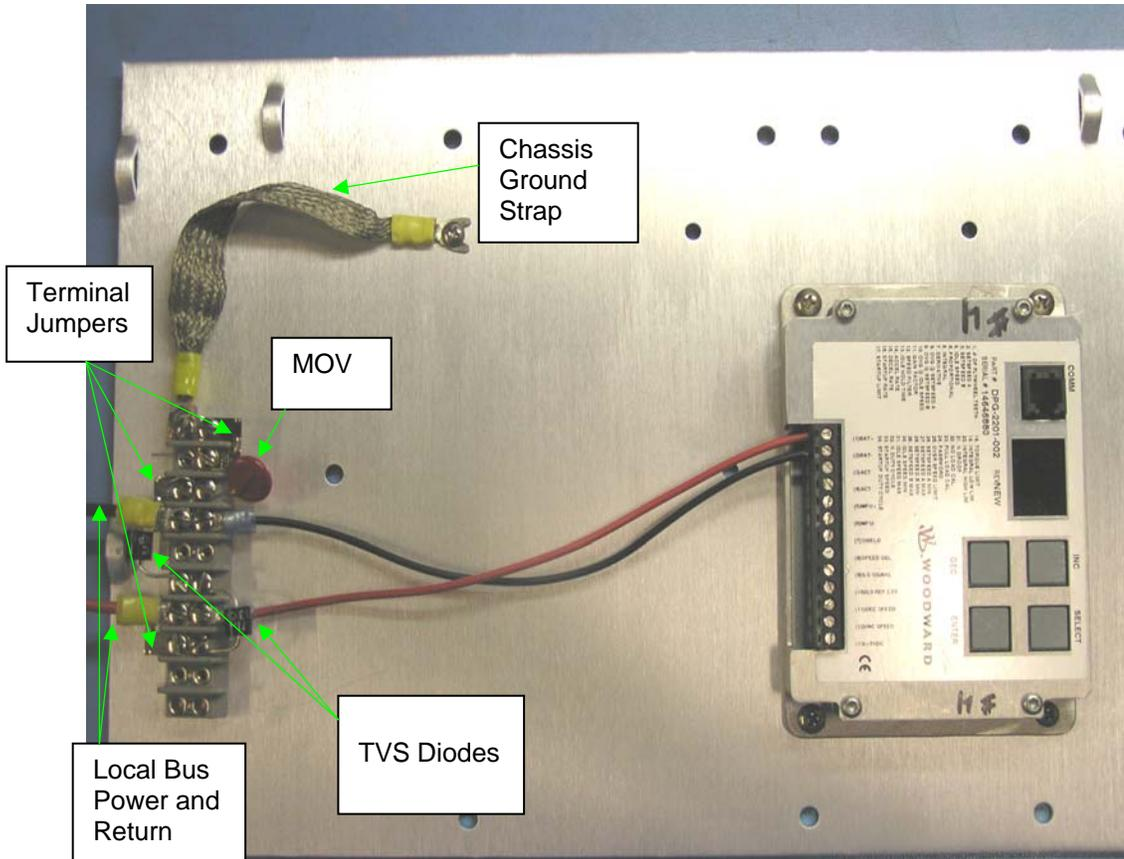
Figure 2. Wiring Example for Centralized Suppression at the DPG Control
