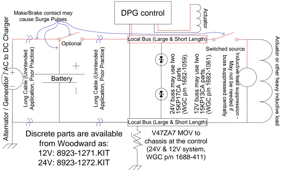
Figure 1. Centralized Suppression Example Implemented at the System Level
