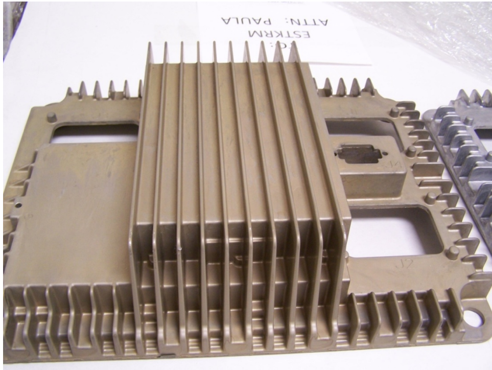
Figure 2. Casting with Yellow Chromate Finish
