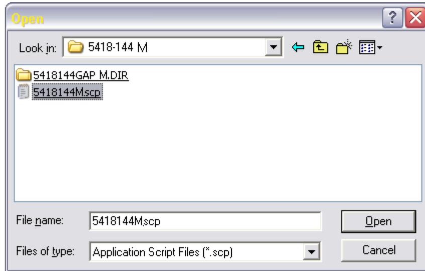
After the Open button is pressed a warning box will appear that tells the user that the control inputs and outputs will be locked during the download. Hit the Yes button to continue. Then a status bar will appear updating the file transfer progress.
