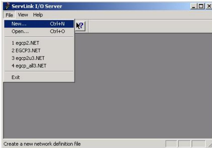
This will open up the Network Options screen. This screen allows the user to configure the ServLink connection for serial com port, or modem. When a serial port is selected, the left side menus will be active and the right side menus will be grayed out.
