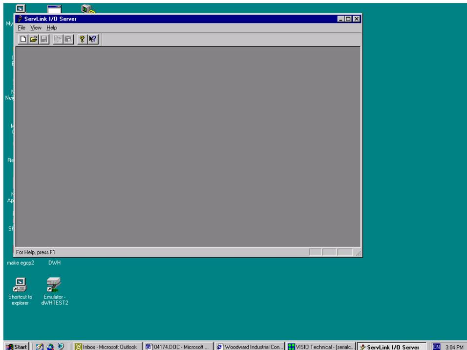
The first action to take inside the ServLink screen is to set up a new network definition file. Click once on File, and then on New as shown. The new network definition window will pop up on the computer screen.
