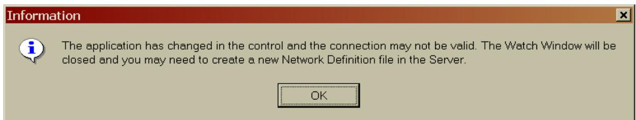
The new software is now loaded in the control. The EGCP-3 should go through a re-boot phase and after about 60 seconds, the screen should show valid data. The software can be verified by going to the password screen of the EGCP-3. On the bottom line of this display the software version is displayed. The software should now be 5418144M.
