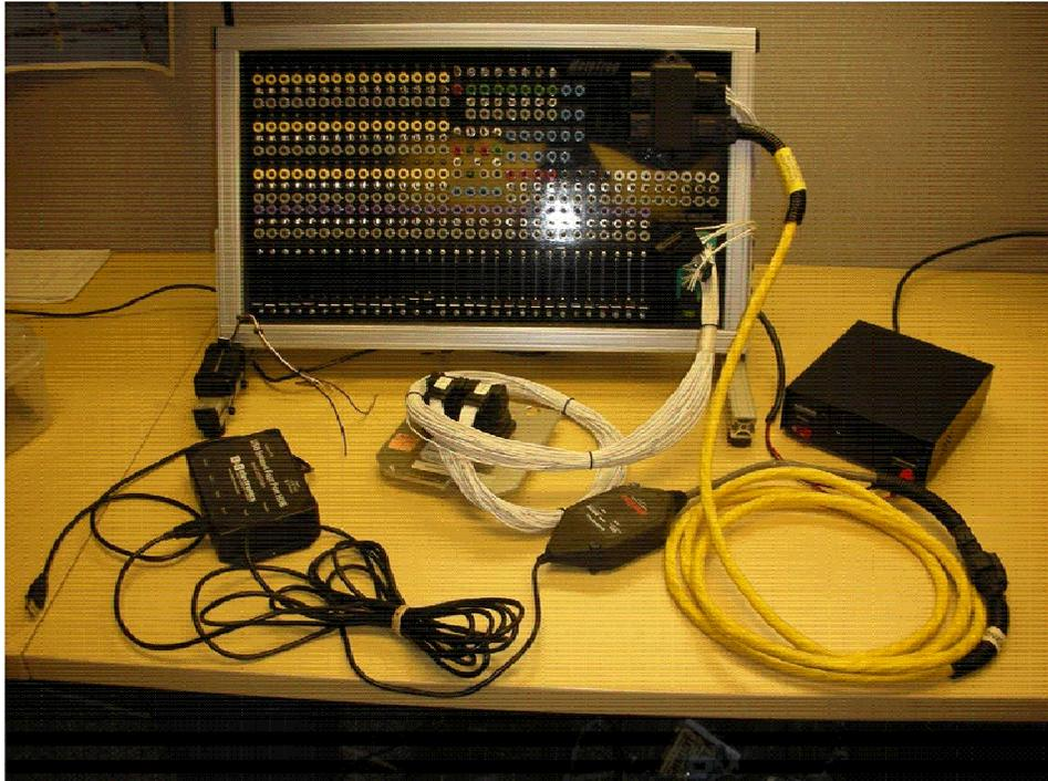
Figure 3-2. Example Desktop IO Simulator Setup
