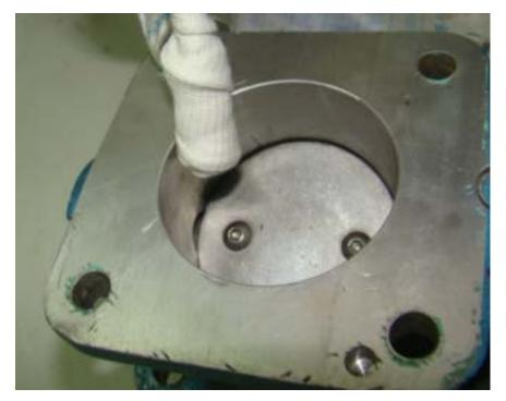
Figure 7. Final Cleaning the Bore with the Cloth Wrapped Bottle Brush
