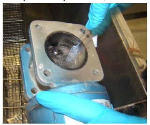
Figure 4. Using Plastic Bottle Brush to Clean Bore
