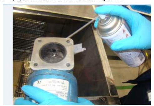
Figure 3. Spraying Solvent into Throttle Bore
