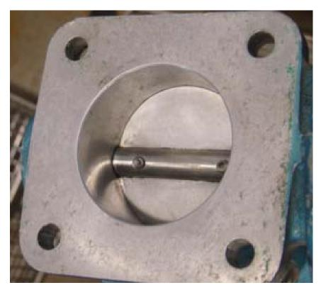
Figure 9. Bore and Plate After Cleaning – Bottom
