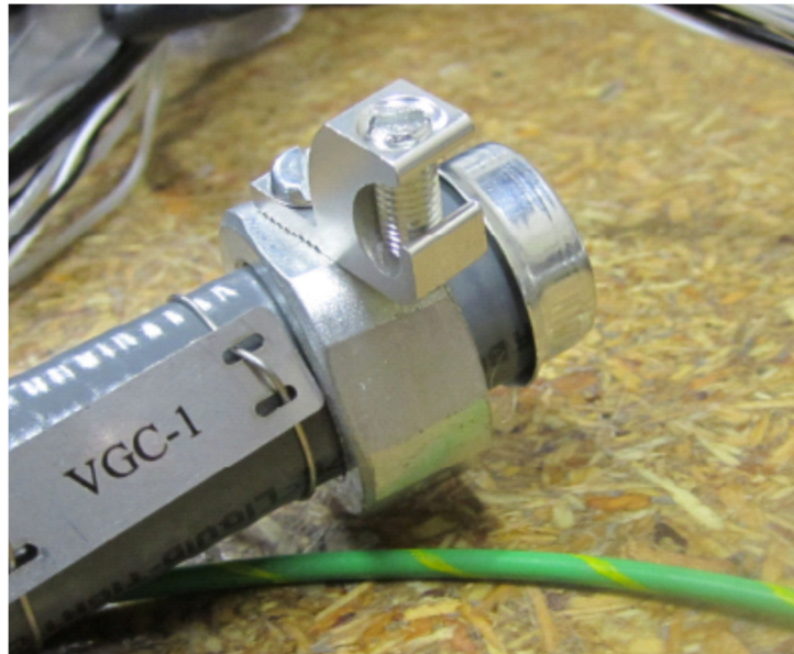
Figure 3-3. Tefzel Grounding Lug
