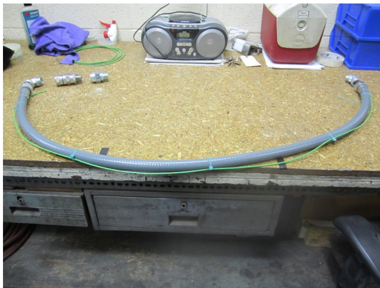
Figure 3-2. Tefzel Grounding Wiring Installation
