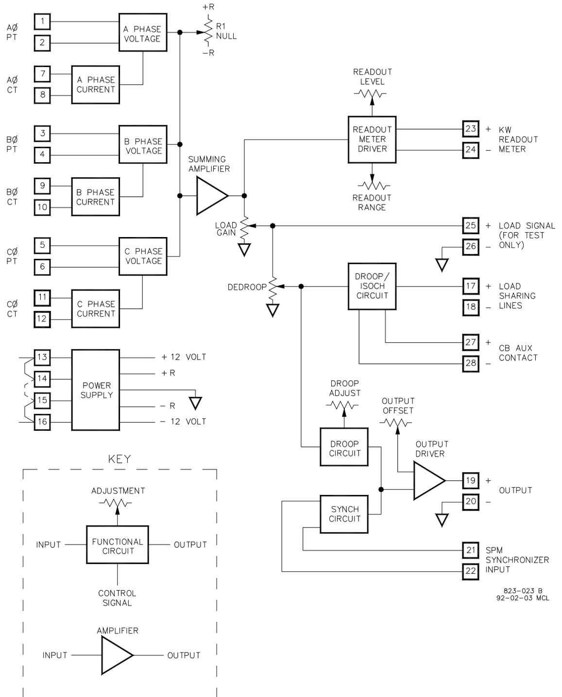
Figure 2-1. 8272-695 Real Power Sensor Block Diagram
