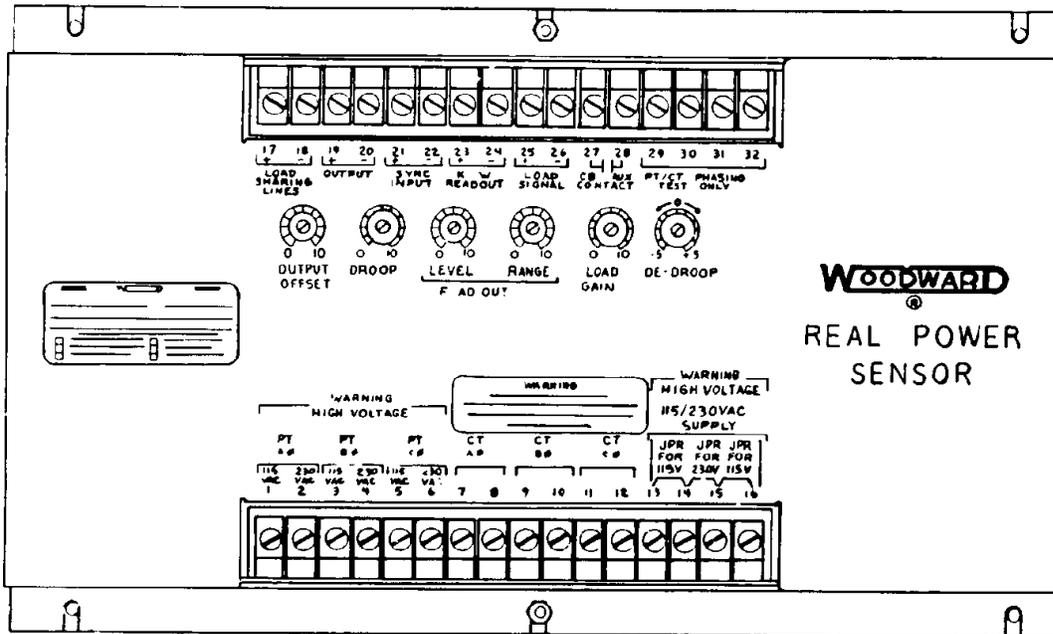
Figure 1-1. 8272-695 Real Power Sensor
