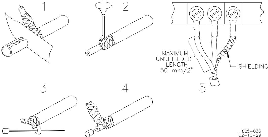
Figure 2-1. Preparation and Installation of Shielded Cables
