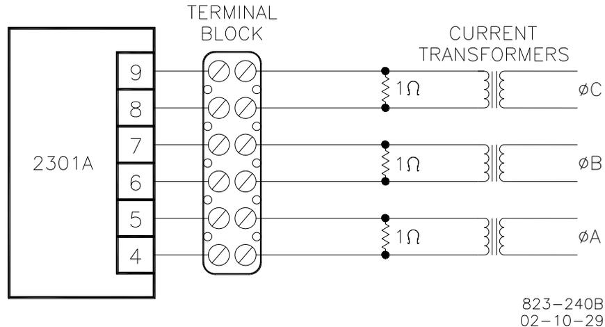
Figure 3-2. Temporary Wiring for Transformer Phase Correction
