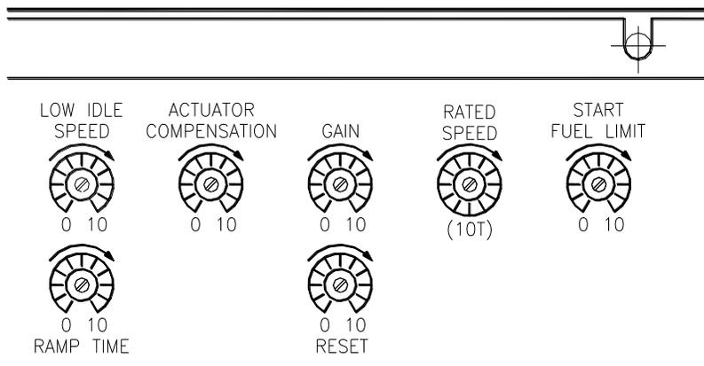
Figure 4-2. Speed Control Adjustments
