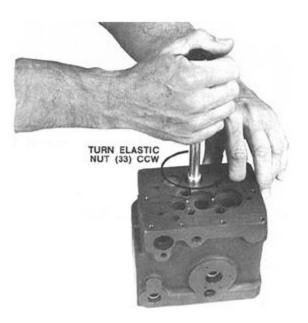
Figure 5-17e. Removing Play in Assembly
