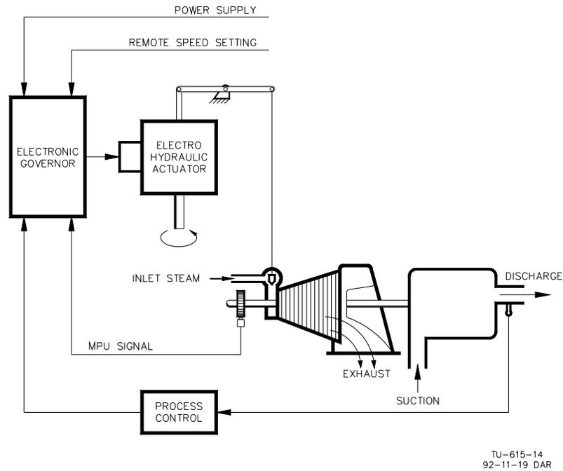
Figure 14. Remote-Process Control
