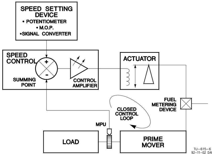
Figure 6. Closed-Loop Control
