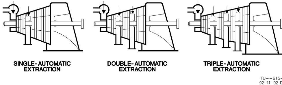
Figure 8. Extraction Turbine
