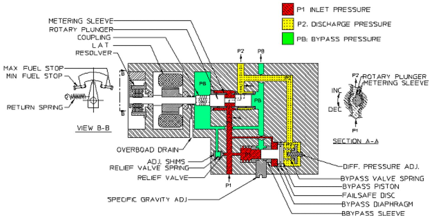
Schematic Diagram – ELV Liquid Fuel Valve
