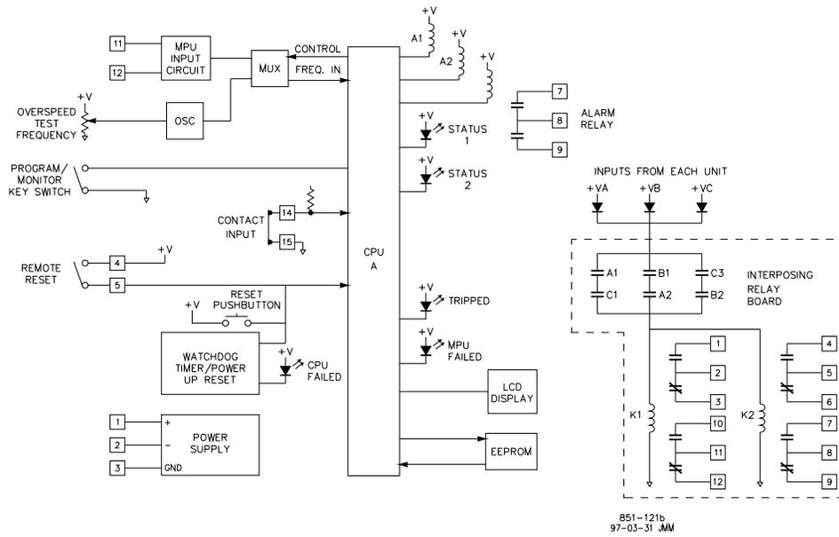
Figure 3-4. Block Diagram of One Unit of ProTech 203 System
