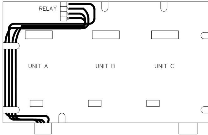
RELAY BOARD FIELD WIRING
