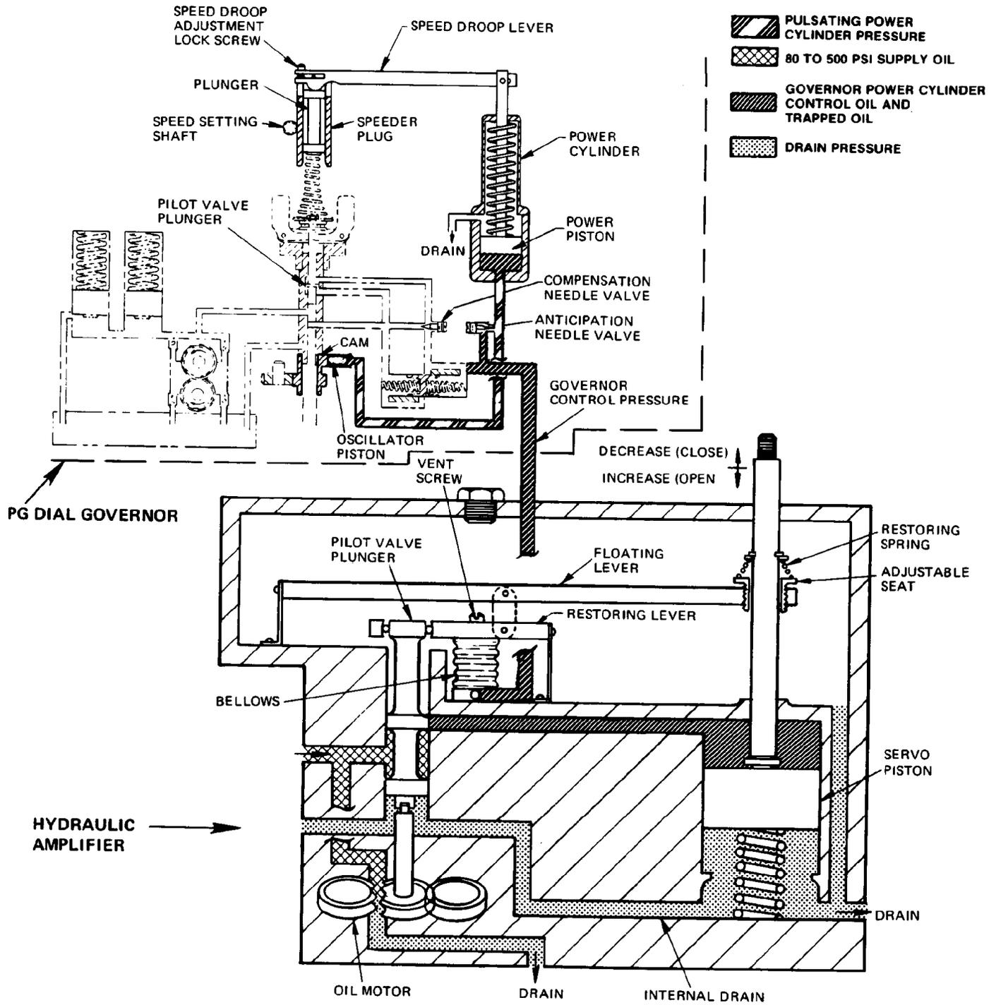
Figure 3-1. Old Type Hydraulic Amplifier (Single Acting) Schematic Diagram
