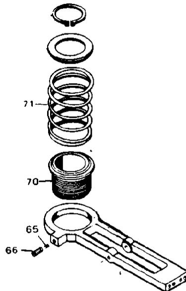
Figure 2-1. Restoring Spring Seat Adjustment
