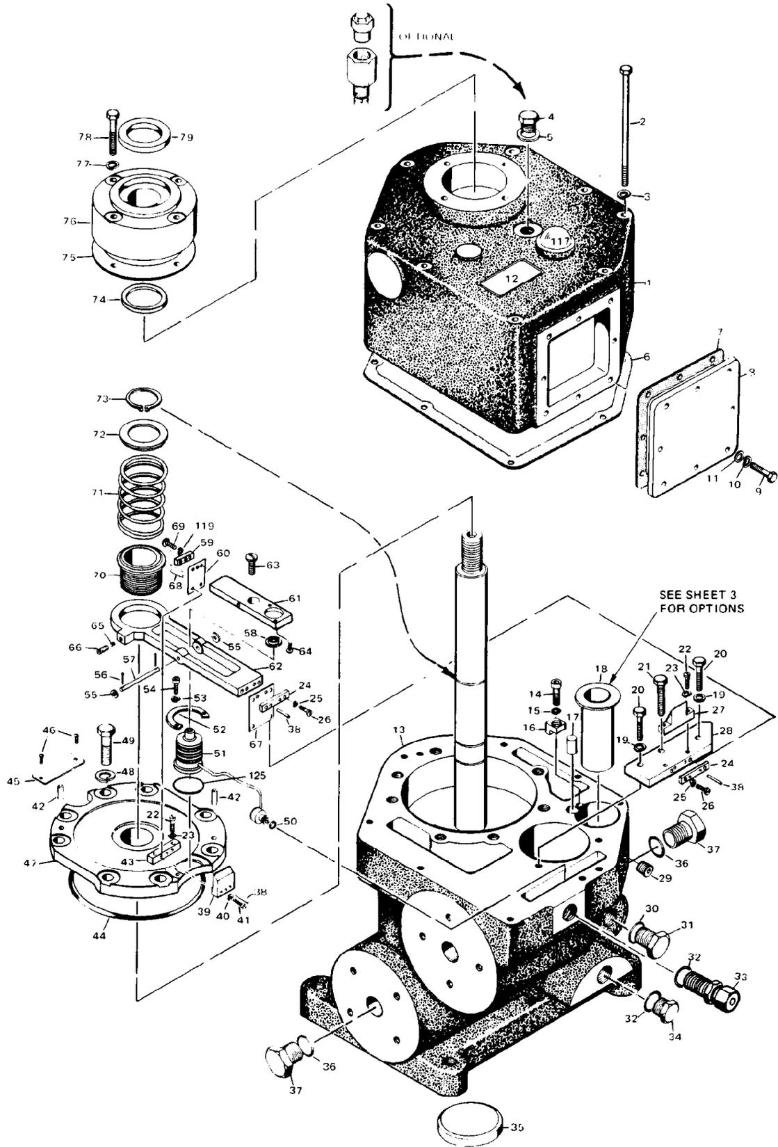
Figure 5-1a. Exploded View of the Hydraulic Amplifier
