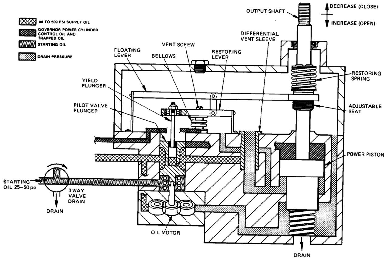
Figure 3-3. Schematic Diagram of the Hydraulic Amplifier with Yield Plunger
