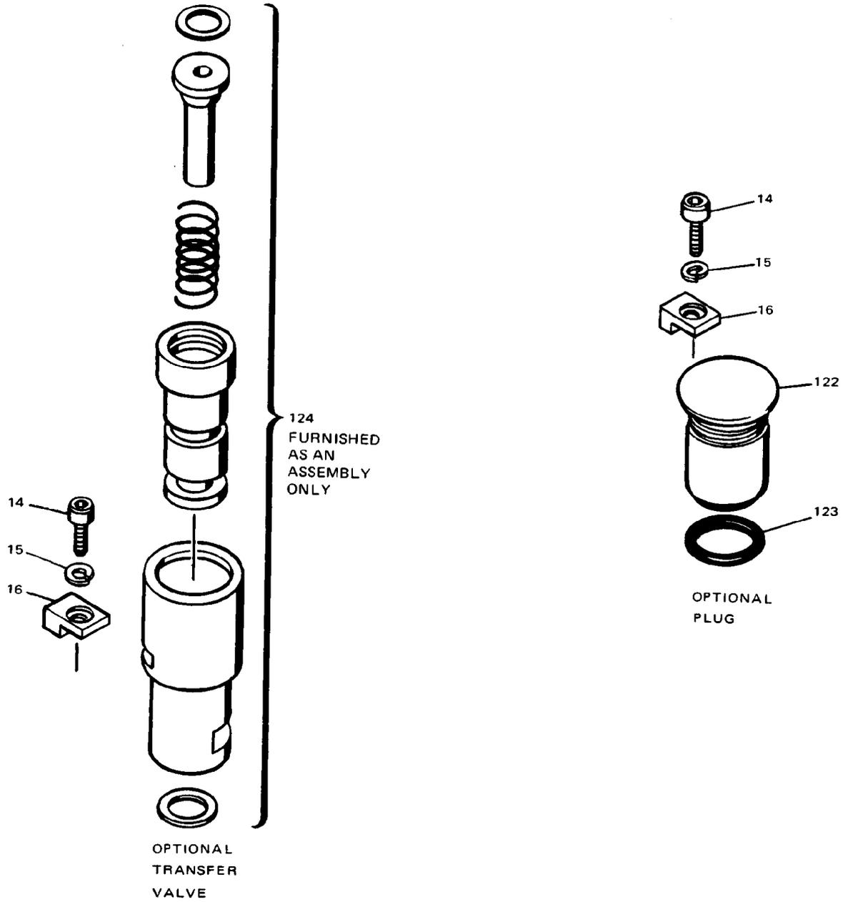
Figure 5-1c. Exploded View of Optional Plug and Transfer Valve Assembly
