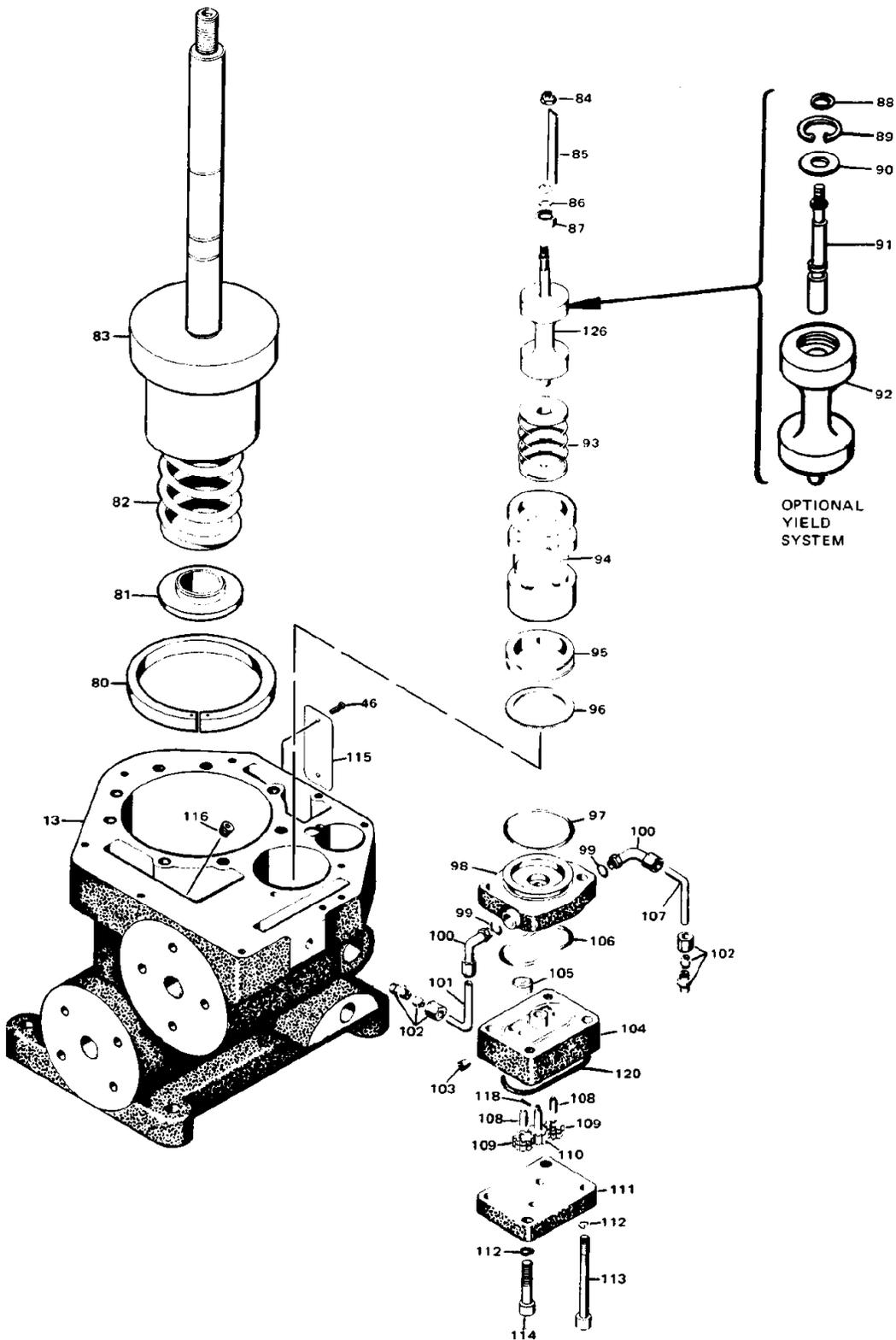
Figure 5-1b. Exploded View of the Hydraulic Amplifier
