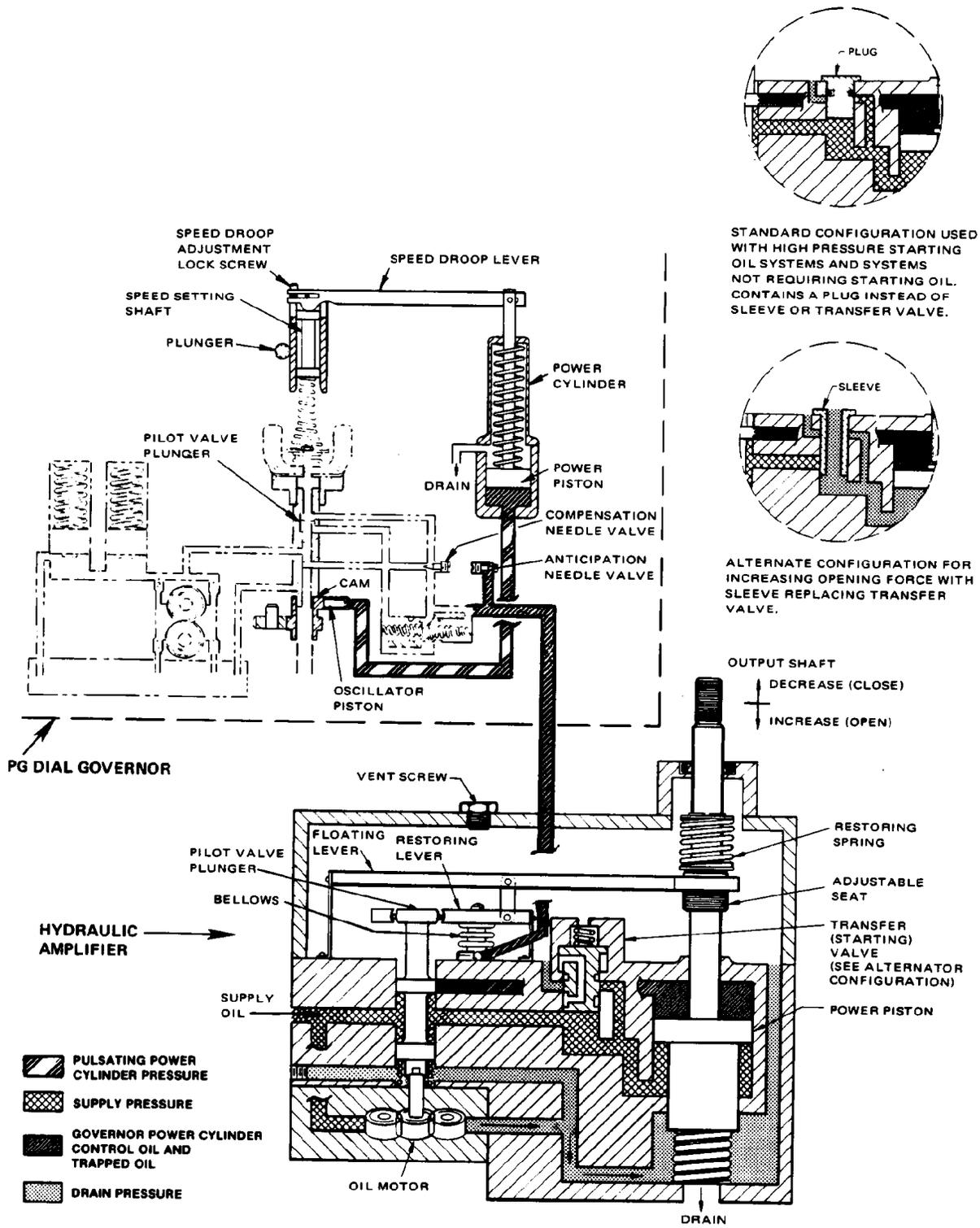
Figure 3-2. Hydraulic Amplifier (Double acting) Schematic Diagram
