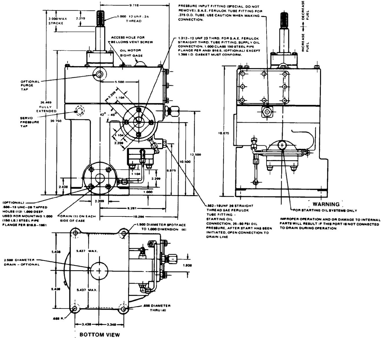
Figure 1-2. Outline Drawing of 7-1/4" Pressure Input Hydraulic Amplifier
