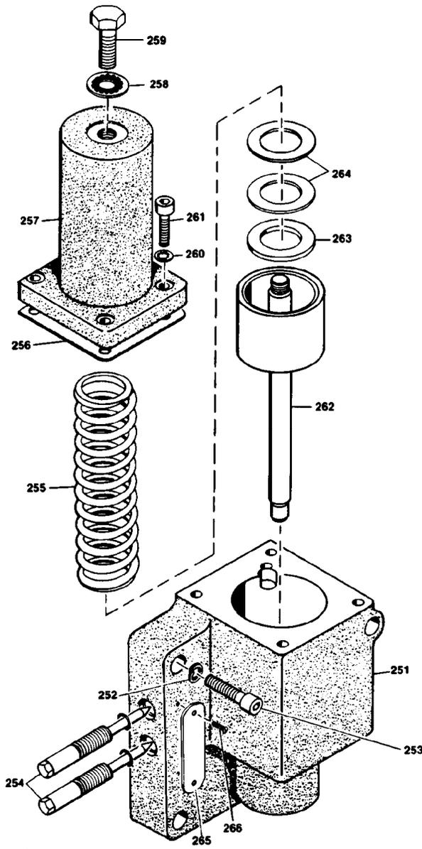
Figure 5-3. Exploded View of the Power Cylinder for a PG-PL Governor
