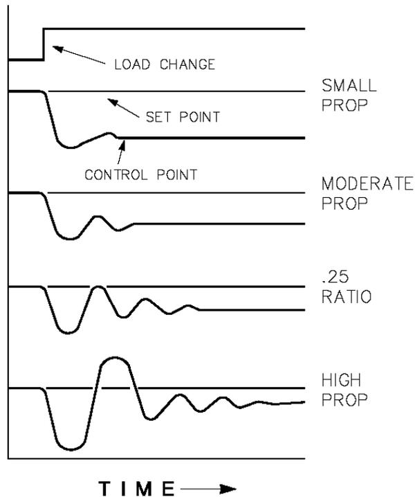
Figure 3-3. Effect of Proportional Gain Settings on Control
