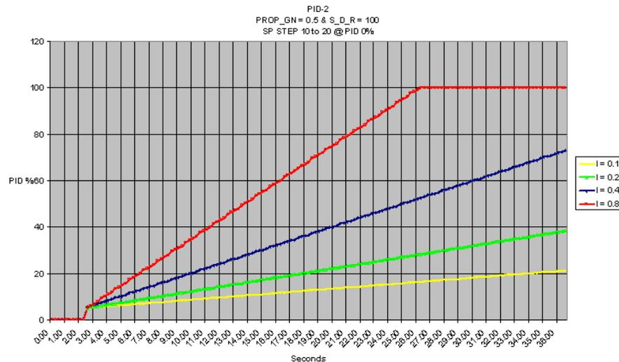
Figure 3-6. Integral Action when Using a Fixed P-gain and no Derivative
