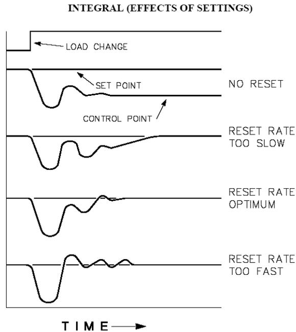
Figure 3-5. Effect of Integral Action on Control
