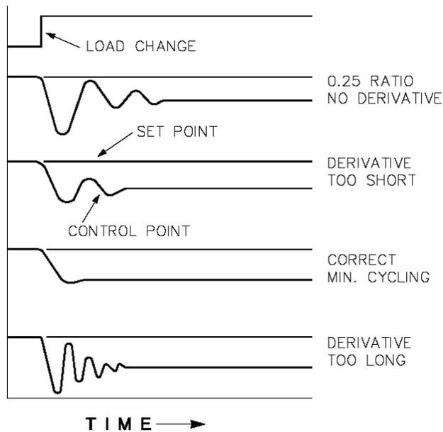
Figure 3-7. Effect of Derivative Action on Control
