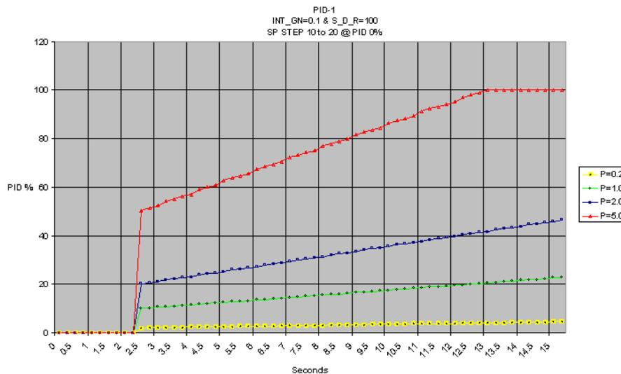
Figure 3-4. Proportional Gain with Fixed Integral and Derivative
