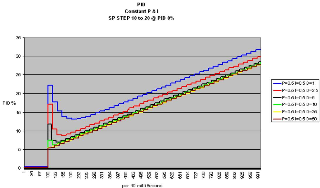
Figure 3-8. Derivative with Fixed Proportional Gain and Integral Action
