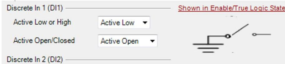
*Active Low, Active Open means it will be detected true when unconnected (or pulled high) and false when pulled low.*
