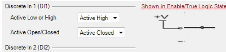
*Active High, Active Closed means it will be detected true when pulled high and false when unconnected (or pulled low).*
