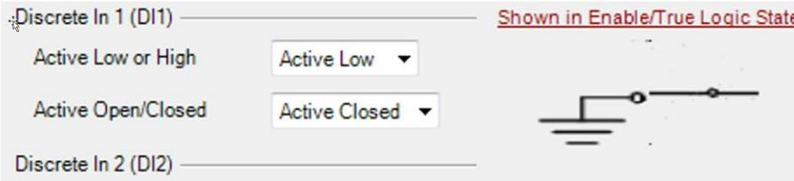
*Active Low, Active Closed means it will be detected true when pulled low and false when unconnected (or pulled high).*
