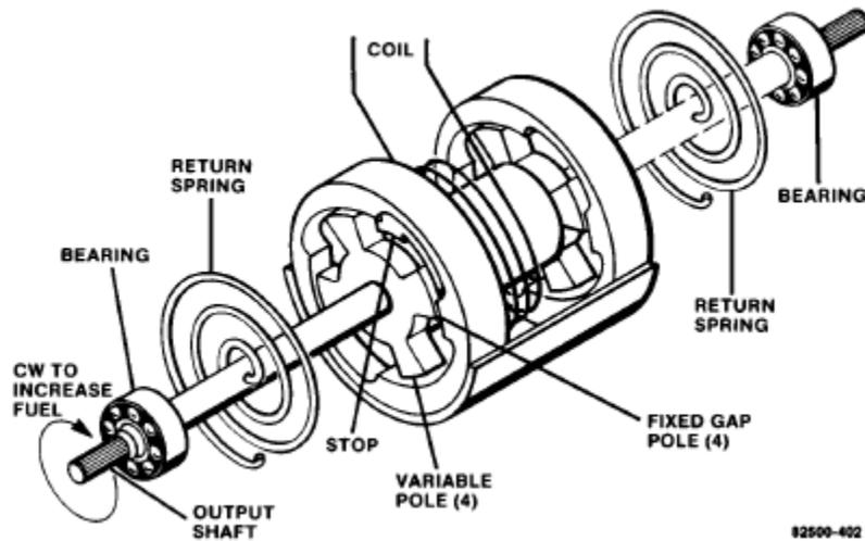
Figure 4-2. Actuator Schematic
