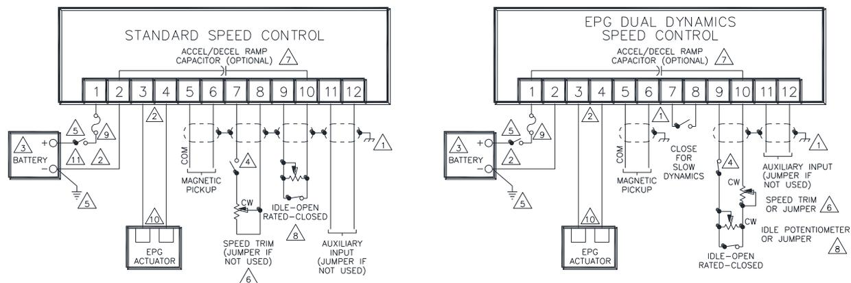
EPG SPEED CONTROL PLANT WIRING
